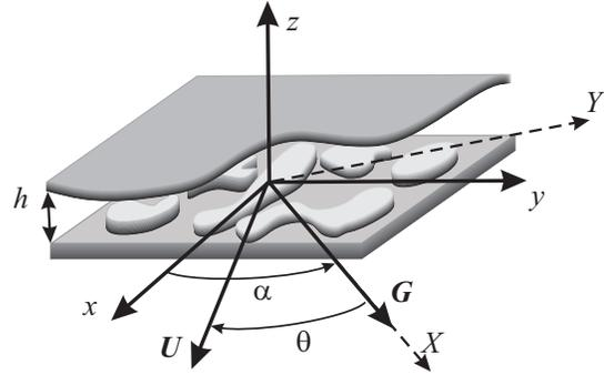
FIG. 1: Sketch of a thin channel of thickness  $h(x, y)$  with notation for directions along the plates. In the Wenzel state the liquid would conform the solid surface, but in the Cassie state it remains free-standing at the top of the roughness
