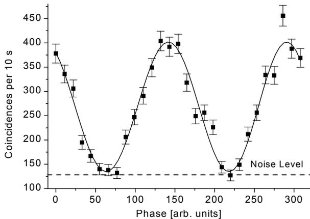
FIG. 2: Experimental data gathered in [8]: “Coincidence counts per 10 s” measures  $P(a = b = 1|\Phi(l_A, l_B))$  for different phase values  $\Phi(l_A, l_B)$ . The dashed line indicates the noise level. The visibility  $V$  after subtraction of the noise is  $97 \pm 5\%$ .
