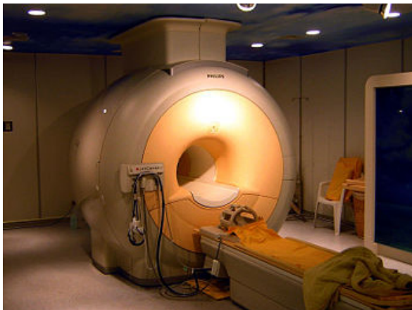
Figure 7. (Left) Modern MRI machine, a large electromagnet (axial magnetic field) with lots of fancy r.f. and computing power. (Right) Typical MRI picture of the head—examination of the brain and other delicate internal parts of the human body without surgery and with exquisite resolution.
