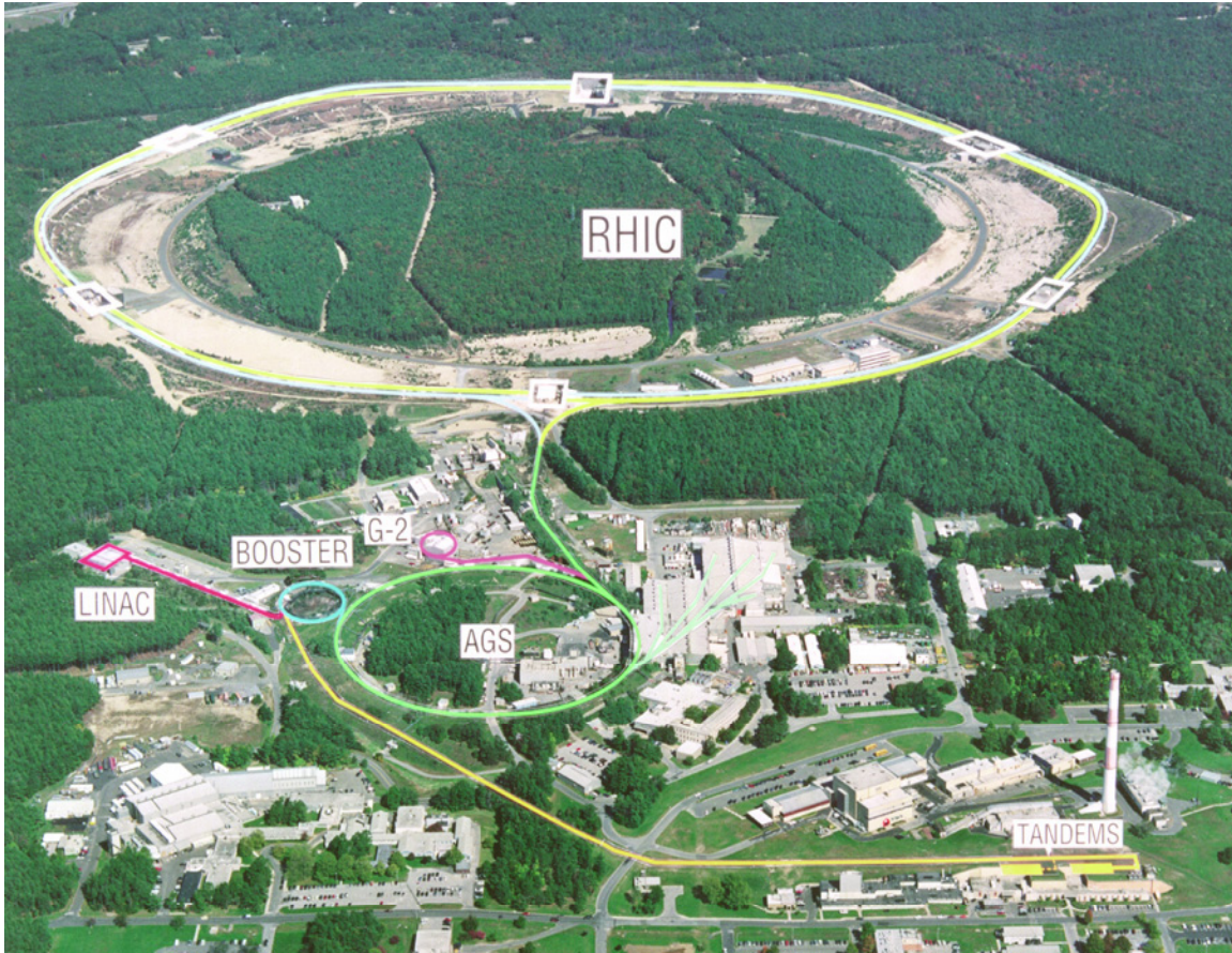
Figure 10. A closer view of RHIC at Brookhaven National Laboratory. The large circle without tree cover is excavation related to the tunnel containing the RHIC machine. The colored lines show the Linac, Booster accelerator for polarized proton injection, the tandem van de graaf accelerator and transfer line to the booster, and the AGS which accelerates the beams to an energy of 22 \text{ GeV per nucleon} \times Z/A where Z and A are the atomic number and weight of the nucleus.
