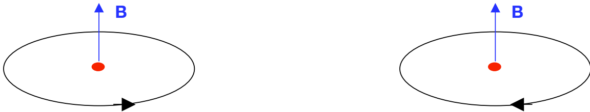
Figure 3. In an external magnetic field, B , the orbit of an electron with 1 unit of angular momentum can only take discrete orientations with respect to the magnetic field.
