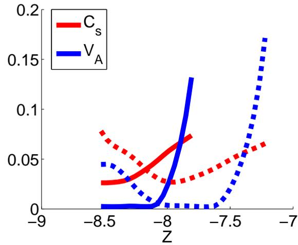
**Figure 3.** (Color online) Alfvén ( $V_A$ ) and ion acoustic ( $C_s$ ) speeds calculated using local plasma parameters at  $t = 15$  (solid lines) and  $t = 20$  (dashed lines), for the case of Table 1.
