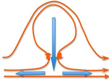
**Figure 5.** (Color online) Schematic of the magnetic configuration around  $t = 20$ . Solid orange lines indicate magnetic field lines, while solid blue arrows indicate internal jet plasma flows (in jet frame of reference). Opposing orange arrows indicate anti-parallel magnetic field where reconnection occurs.
