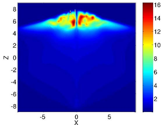
**Figure 8.** (Color online) Density in the  $X$ - $Z$  plane with  $Y = 0$  at  $t = 25$  ( $8.53 \mu s$ ) for NSTX-relevant parameters of Table 2, showing deep jet penetration. The density structure seen here is characteristic of early time evolution likely due to internal jet mass flow induced by reconnection at the tail. The density smooths out at later times which is the case in Fig. 6.
