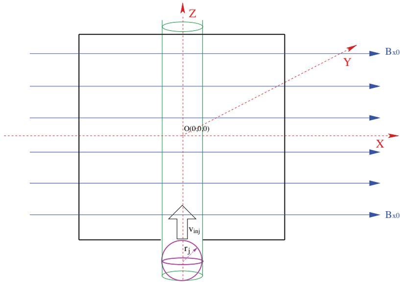
**Figure 1.** (Color online) Schematic of the simulation geometry showing the coordinate system, the background magnetic field, the injected plasma (with spherical radius  $r_j = 0.5$ ), and the background plasma (cubic with sides of length = 18).
