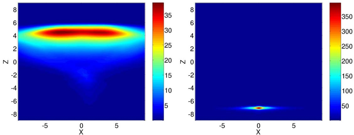
**Figure 6.** (Color online) (*left*) Density contours at  $Y = 0$  and  $t = 150$  for parameters of Table 1, showing deep but not highly localized deposition. The jet is still moving at nearly the initial injection speed. (*right*) Density contours at  $Y = 0$  and  $t = 80$  with the same parameters except  $v_{inj} = 0.056$  (93.3 km/s), showing shallow but more localized deposition. Note that the color scales are not identical.
