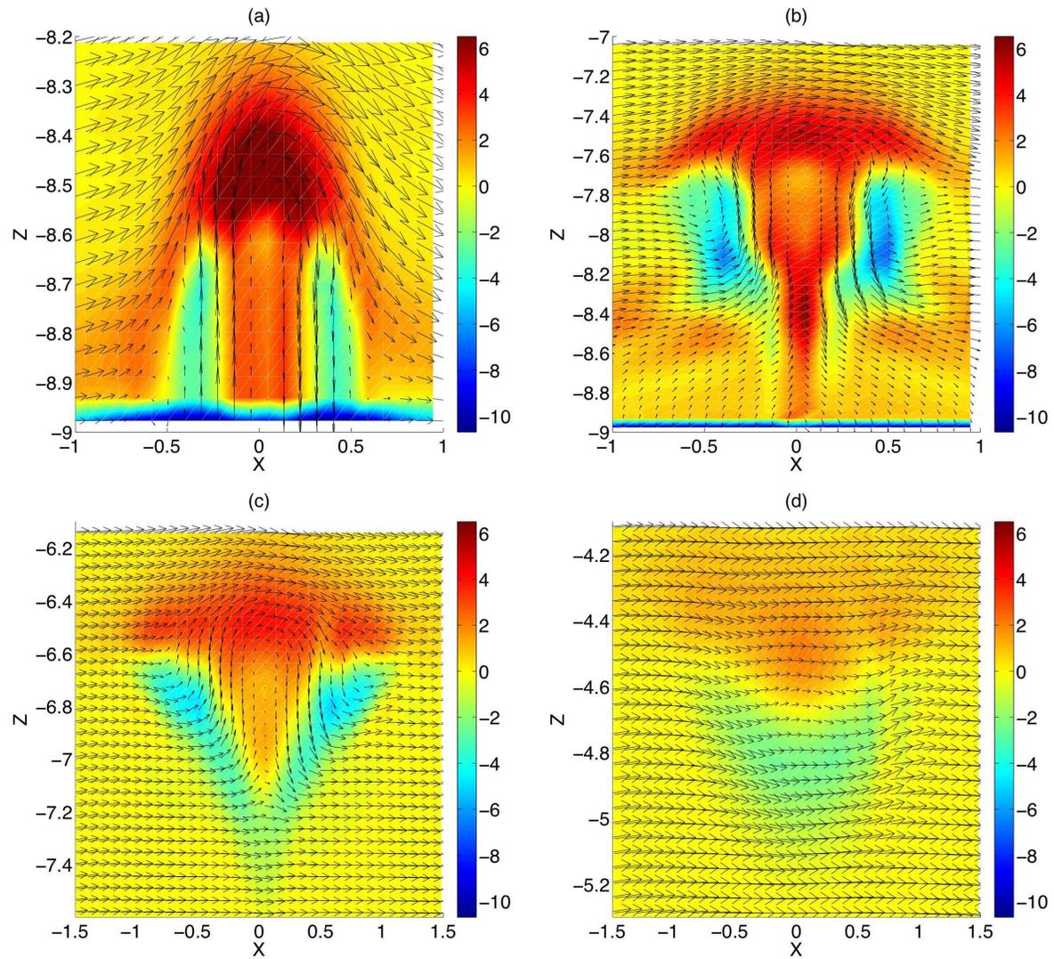
**Figure 2.** (Color online) Contours of  $j_y$  and vectors of  $\vec{B} = (B_x, B_z)$  for parameters of Table 1: (a)  $t = 10$  ( $0.59 \mu\text{s}$ ), (b)  $t = 20$ , (c)  $t = 30$ , (d)  $t = 50$ . Note that the scales for the abscissa and ordinate are not identical.
