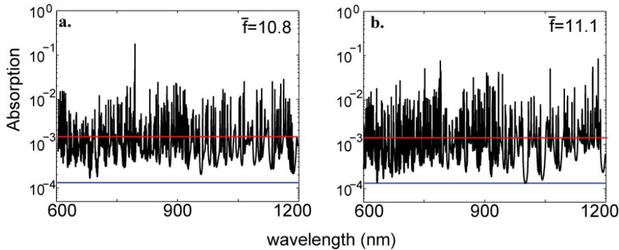
Fig. 4. Absorption spectra for off-normally incident light (averaged among s and p lights). Light incidence angle is  $30^\circ$  and incident plane is oriented at azimuthal angle  $30^\circ$ . a) for the asymmetrical structure in Fig. 1a. b) for the symmetrical structure in Fig. 3a.
