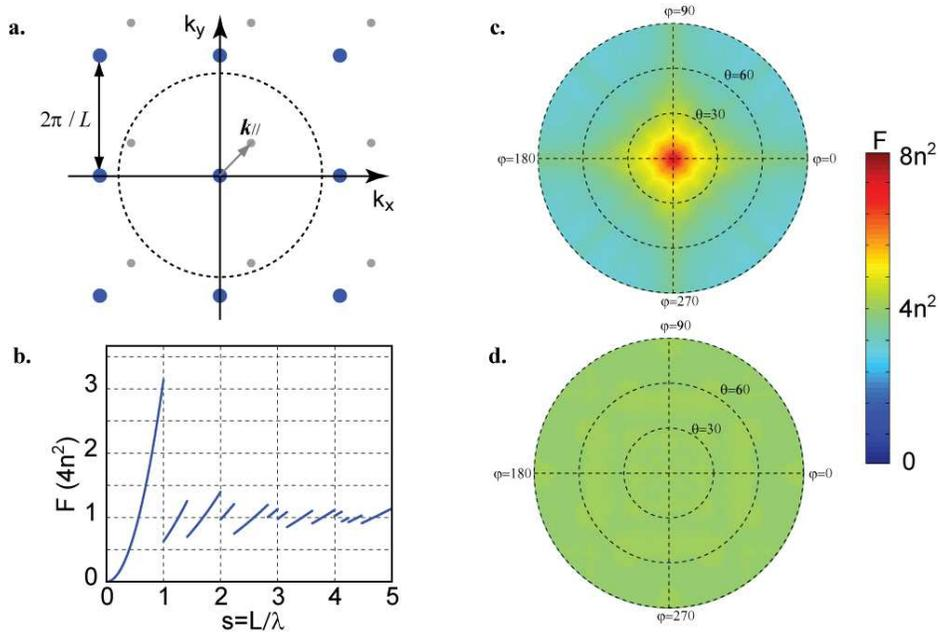
Fig. 5. a) Channels in 2D  $k$ -space. Blue and grey dots represent channels when the incident light comes in from normal and off-normal directions, respectively. The radius of the circle is  $k_0$ . b) Limit of absorption enhancement in 2D grating structures. c) Angular response of the average enhancement factor integrated over wavelength from 600nm to 1200nm. The periodicity of the grating is 600nm. d) the same as (c) except the periodicity is 3000nm.
