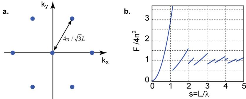
Fig. 7. a) Channels in 2D  $k$ -space for a grating with triangular lattice periodicity. The lattice constant is  $L$ . b) Upper limit of absorption enhancement for gratings with triangular lattice periodicity.
