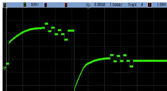
Figure 16: The voltage output of 8 columns multiplexed.
