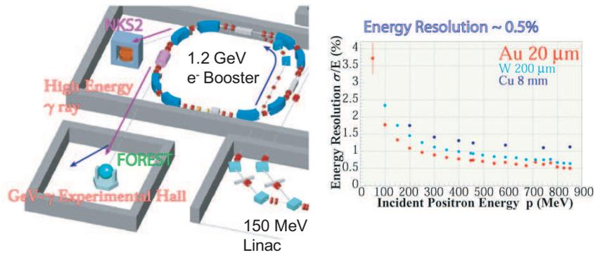
Figure 3: Layout of the Tohoku LNS accelerator facility (right). Users area is located in GeV- $\gamma$  experimental hall in the picture. Left plot is the energy spread of the positron beams for different types of gamma-conversion target.
