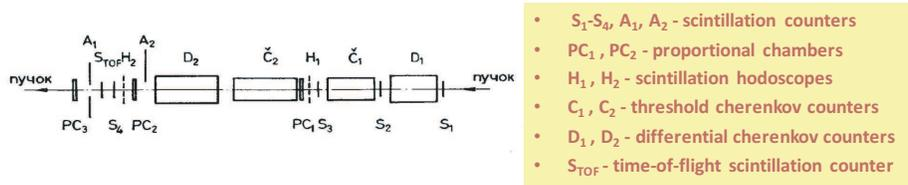
Figure 6: Layout of one of the beam lines (N2B) at IHEP Protovino in Russia.
