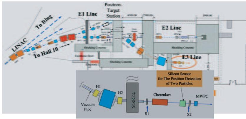
Figure 4: Schematic view of the test beam area in IHEP at Beijing.
