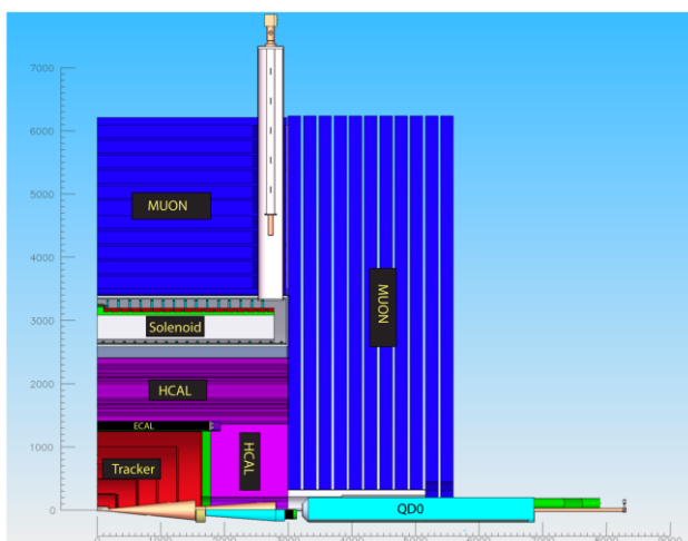
Figure 1. Quarter section view of the SiD detector.
