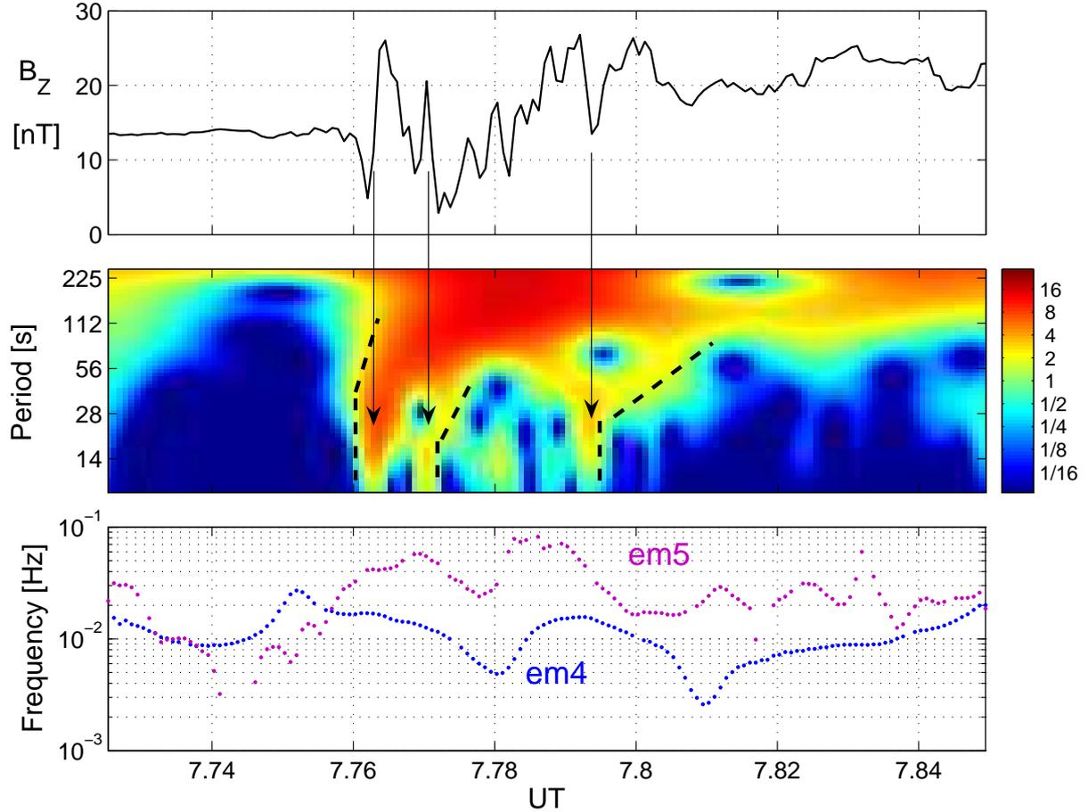
**Fig. 4.** Top: magnetic field time series; Middle: Wavelet time-period-energy representation; Bottom: Hilbert-Huang time-instantaneous frequency representation; Thick dashed lines in the middle indicate the wavelet time-scale evolution in time; Line arrows show the locations of short time-scale (high-frequency) activations occurring simultaneously with the largest jumps in  $B_Z$ .
