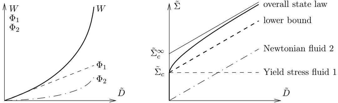
Figure 10: One-dimensional sketch of the functions  $W$ ,  $\Phi_1$  and  $\Phi_2$  as a function of the second invariant of  $\mathbf{D}$  (left). The associated state laws (fictitious materials, lower bound and overall material) are depicted on the right part of the figure. The suspending fluid is Bingham ( $n = 1$ ).
