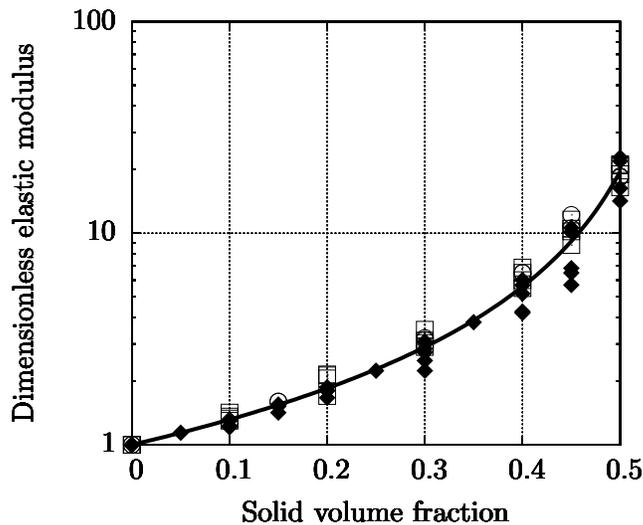
Figure 4: Dimensionless elastic modulus  $G^{\text{hom}}/G$  vs the beads volume fraction  $\varphi$  for all the systems studied by Mahaut et al. (2007). The open square symbols are suspensions of polystyrene and glass beads in bentonite, the open circle symbols are suspensions of glass beads in carbopol while the solid diamond symbols are suspensions of polystyrene and glass beads in emulsion. The solid line is the Krieger-Dougherty Eq. (23) with  $\varphi_m = 0.57$ .
