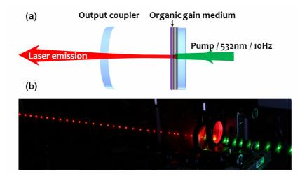
Figure 1 – a) Schematic representation of the plano-concave VECSOL resonator (see text for details). b) Long-exposure time photo of the working VECSOL.
