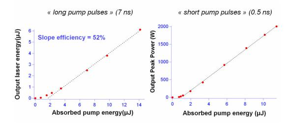
Figure 2 – Output laser energy (left) and output peak power (right) vs. absorbed pump energy inder 7 ns and 0.5 ns pumping, respectively. The dashed line is a linear fit to the experimental lata.
