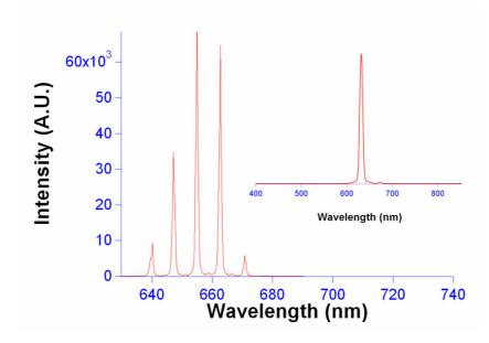
Figure 3– Typical emission spectrum of a 17- $\mu$ m thick active layer. Inset: single peak lase peration achieved for a 2.35- $\mu$ m layer.
