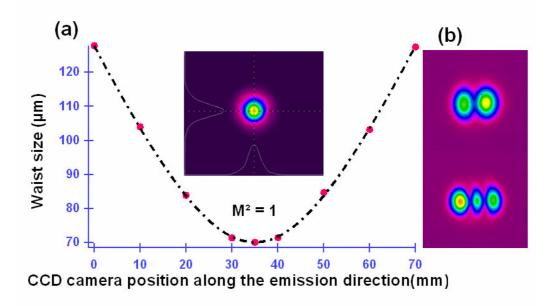
Figure 3 – a) Spatial evolution of the output beam profile along the emission direction. The dotted line is a fit to the experimental data with  $M^2=1$ . Inset: TEM<sub>00</sub> laser beam profile. b) TEM<sub>10</sub> and TEM<sub>20</sub> images of the VECSOL emission obtained by fine misalignment of the VECSOL cavity.
