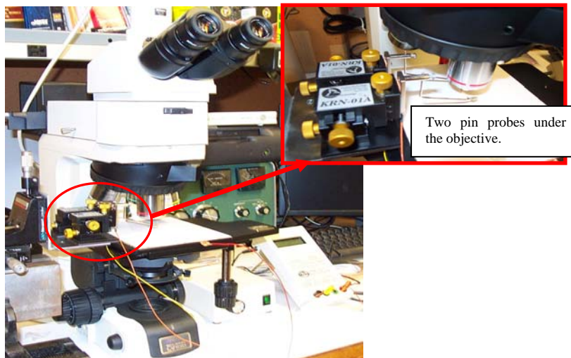
Fig. 8. Nikon microscope and two pin-probes with their 3D micrometer stages (the insert shows two pin-probes).
