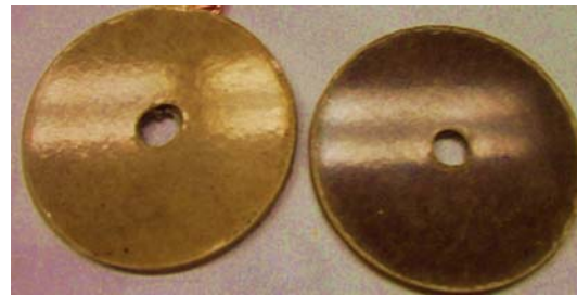
Fig. 14. The left disc is high dose sample, it shows discolored “orange peel” like surface, the right disc is low dose sample, its surface looks reasonably smooth and darker.
