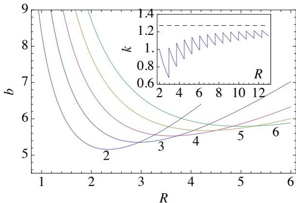
FIG. 2: Monotonic instability thresholds for a circular droplet of radius  $R$ . The numbers indicate the value of  $n$ . Instability occurs above the lower envelope of the family of curves. Inset: the wavenumber  $k = n/R$  for the most dangerous mode; the dashed line indicates the respective value for the rectilinear contact line.
