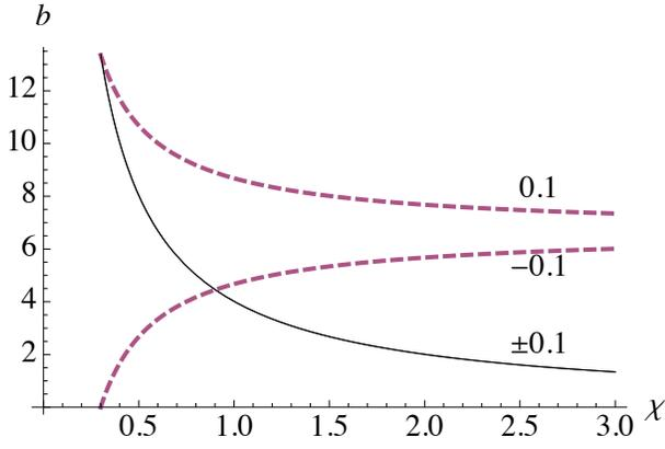
FIG. 4: Loci of monotonic (dashed lines) and oscillatory (solid line) instability in the parametric plane  $\chi, b$  for the rectilinear contact line moving with the speed  $u = \pm 0.1$  (as indicated by numbers at the curves). The stable domain is in below both respective curves.
