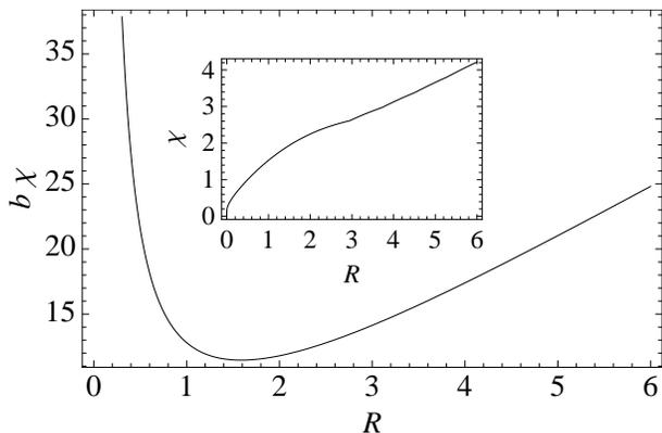
FIG. 3: The lower limit of the product  $b\chi$  at the traveling instability limit as a function of radius  $R$ . Inset: The lower limit  $\chi_t$  at which the traveling instability precedes the monotonic one.
