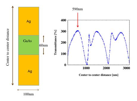
**Fig.9:** Left: GaAs-filled nanocavity 100nm deep and 60nm wide on an infinite array. Departures from these parameters can reduce transmittance and field amplification inside the cavity. Right: Transmittance vs. pitch, normalized to the energy that falls directly on the cavity area. Maxima are Fabry-Perot resonances; minima correspond to Woods anomalies.
