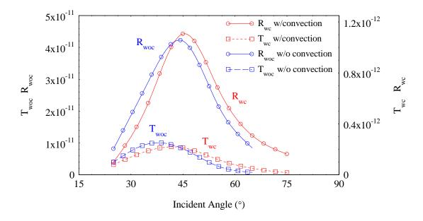
**Fig.6:** TE/TM-incident/TE-detected, reflected and transmitted SH conversion efficiencies, with (right axis) and without (left axis) convection. Convection shifts the peaks to larger angles, but reduces both signals by nearly a factor of 50. The subscript "woc" stands for "without convection", and "wc" stands for "with convection".  $m^* = m_e$ , and  $n_0 = 5.8 \times 10^{22} / \text{cm}^3$ .
