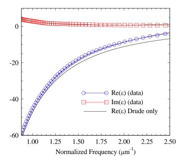
**Fig.1:** Markers: Real and imaginary parts of the dielectric constant of Ag in the 1064-400nm range. The solid curves that retrace the data correspond to Eq.(1). The lower solid curve that runs below all others is only the Drude portion of Eq.(1).
