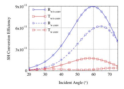
**Fig.5:** TM-incident/TM-detected, reflected and transmitted SH efficiencies, with and without convection. Convection shifts and reduces the amplitude of the reflected signal, while turning the transmission maximum into a minimum. The subscript "w/o" stands for "without", while the subscript "w" stands for "with". We have assumed that  $m^* = m_e$ , and  $n_0 = 5.8 \times 10^{22} / \text{cm}^3$ .
