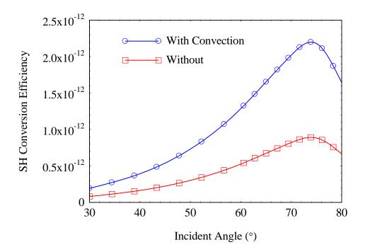
**Fig.3:** Conversion efficiency for TM-incident (1064nm)/TM-detected (632nm) light for a 125nm-thick silver layer. The effective mass and densities of both free and bound charges are taken to be  $m^* = m_e$ , and  $n_0 = 5.8 \times 10^{22} / \text{cm}^3$ , respectively.
