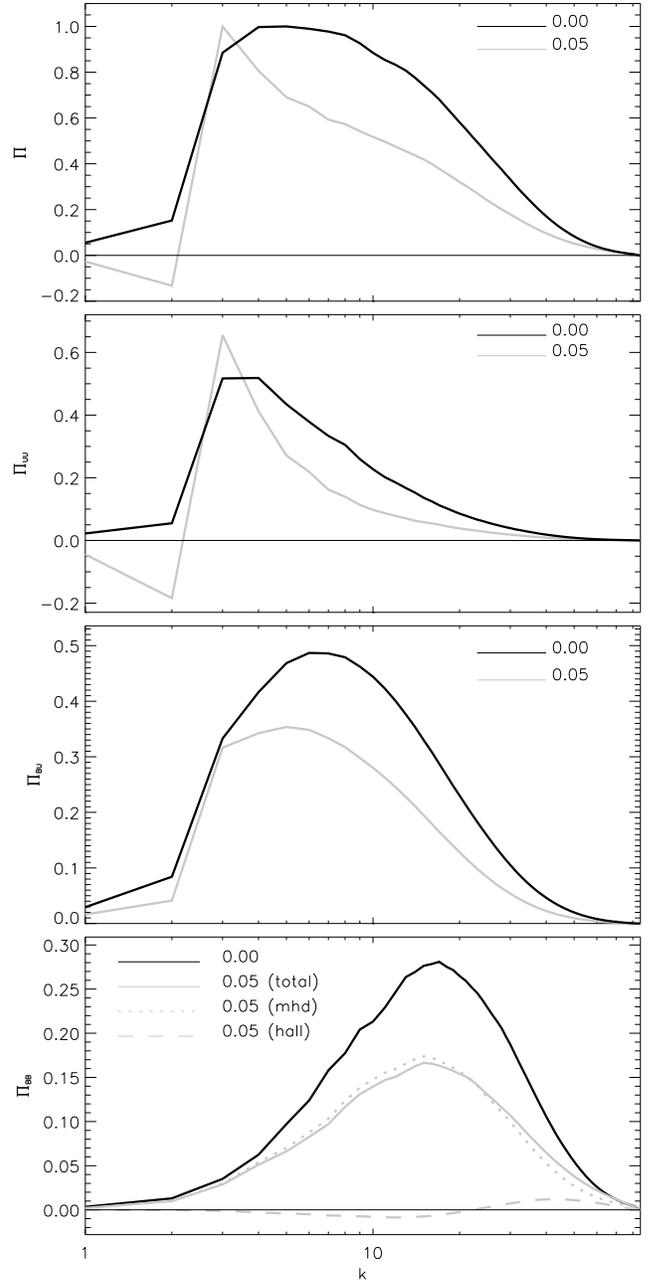
FIG. 8. Energy fluxes vs.  $k$ , normalized by the total dissipation rate  $D$ . The black line corresponds to a time average at the stationary regime of the run with  $\epsilon = 0$ , while the gray line is for  $\epsilon = 0.05$ .
