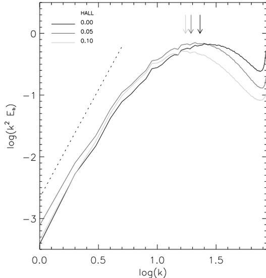
FIG. 6. Spectral distribution of current density, i.e.,  $k^2 E_b(k)$  vs.  $k$  for three different values of the Hall parameter (labeled). The dotted trace corresponds to the Kazantsev slope  $k^{7/2}$ . The arrows indicate the average wavenumber  $k_J$  (see Eqn. 6) for each distribution.
