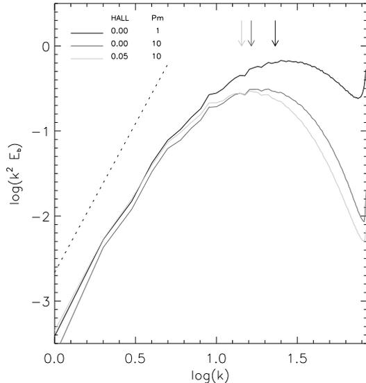
FIG. 11. Spectral distribution of current density, i.e.  $k^2 E_b(k)$  vs.  $k$  for three runs with different values of  $\epsilon$  and  $Pm$  (labeled). The dotted trace correspond to the Kazantsev slope  $k^{7/2}$ . The arrows indicate the average wavenumber  $k_J$  (see Eqn. 6) for each of the current density distributions.
