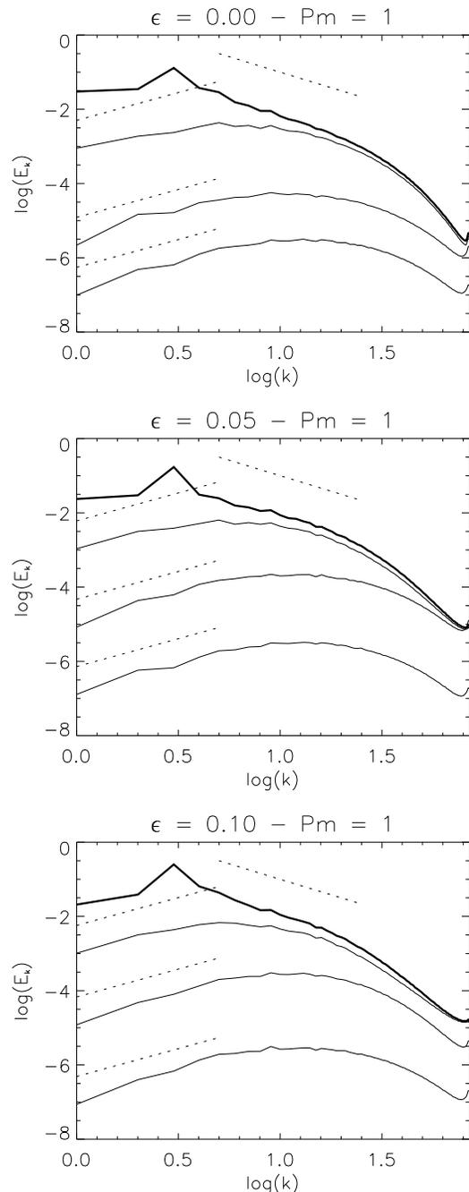
FIG. 5. Total energy spectrum (thick trace) at  $t = 72$  for different values of  $\epsilon$  (labeled). In each frame magnetic energy spectra at  $t = 18, 36, 72$  are also shown (corresponding to the thin lines from bottom to top). The Kolmogorov and Kazantsev spectra are overlaid (dotted trace) for reference.
