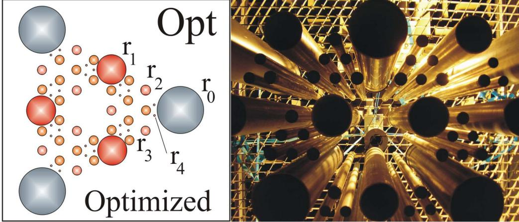
FIG. 2. (Left) Optimized arrangement of scatterers based on Sierpinski triangle with different relationships among the radii of the cylinders ( $QFS_{Opt}$ ); (Right) Photograph taken from beneath the commercial arrangement ( $QFS_{Exp}$ ) used to validate theoretical results. Part of the supporting frame can be seen also.
