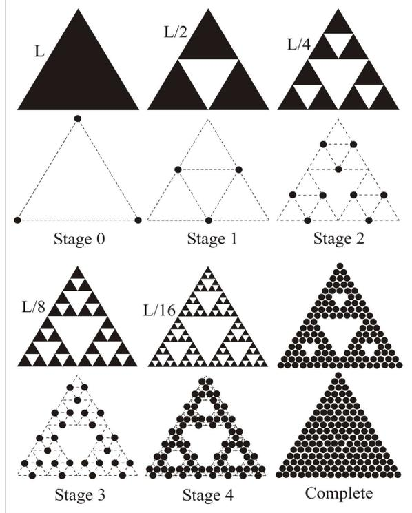
FIG. 1. Quasi fractal arrangement of scatterers: Five stages of cylinder arrays based on the Sierpinski's triangle geometry and the resulting complete structure.
