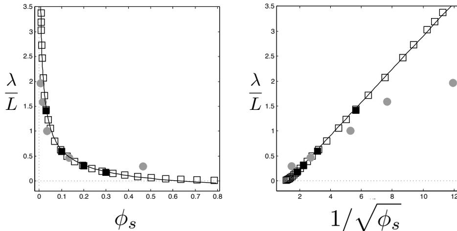
FIG. 2: Results of our model, and comparison with previous computational and experimental work, in the case of a square lattice. Effective slip length,  $\lambda/L$ , as a function of the solid surface fraction,  $\phi_s$  (left), and as a function of  $1/\sqrt{\phi_s}$  (right). Solid line: Simple asymptotic low  $\phi_s$  model, (34); Empty squares: Computations by [27]; Filled squares: Computations by [26]; Filled circles: Experimental results by [25].
