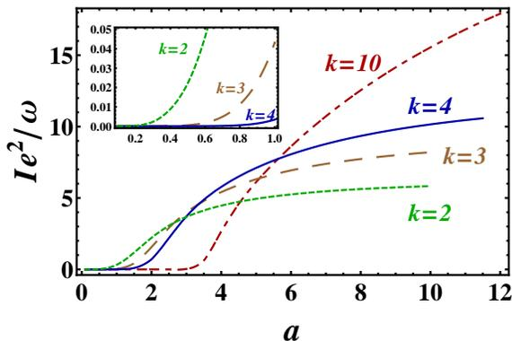
FIG. 7. The net positive/negative current (40) carried by interior/exterior of the vortex with the winding number  $k$  vs the vortex size  $a = e\eta R_{\text{vort}}$ . The inset shows zoom in on the region with  $a < 1$ .
