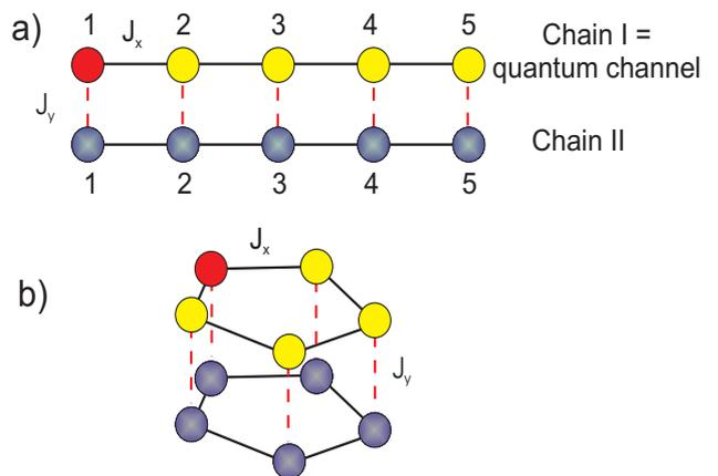
Figure 1: (Color online): (a) Schematic representation of the spin ladder system given by the Hamiltonian of Eq. (1). Each spin chain has  $M = 5$  spins. (b) A system like in (a) but with periodic boundary conditions between spins 1 and  $M$ . Light colors represent the quantum channel. Marked spin (red online) represents the site where the initial condition is placed.
