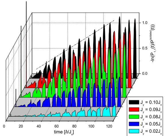
Figure 3: (Color online): Natural logarithm of the ratio  $P_{11}(t)/P_{1,1}^{\text{isolated}}(t)$  for different values of the transversal coupling  $J_y$  as a function of time. The interaction between chains has an isotropic nature. The dashed line is a guide to the eye.
