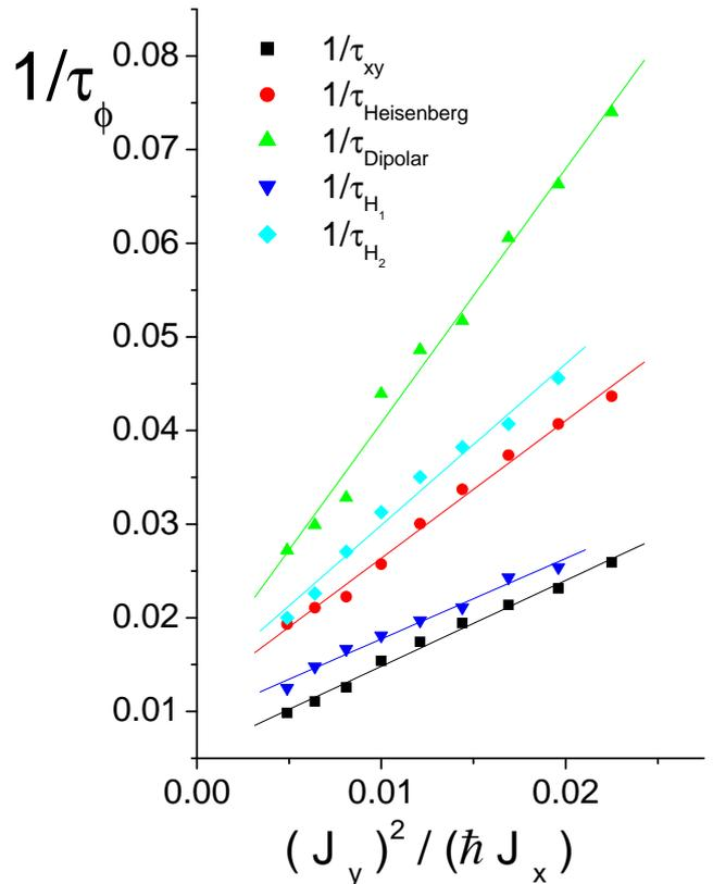
Figure 5: (Color online): Decoherence rates  $\frac{1}{\tau_\phi}$  for different transversal Hamiltonians as a function of  $|J_y|^2/\hbar J_x$ . The linear dependence indicates the good agreement with the FGR behavior. Different slopes indicate that the decoherence rate is composed by two contributions: One is due to the injection of polarization produced by the  $XY$  term of  $\widehat{\mathcal{H}}_T$  and the other is associated to the dephasing process given by the Ising term.
