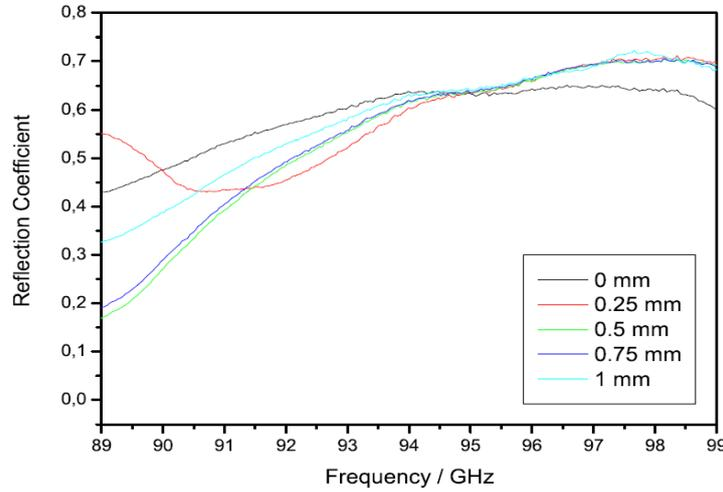
Figure 4. Reflection coefficient measurement at the input port of the mixer mount for different back-short position. A colour version of the graph can be found in the on-line version of the paper.
