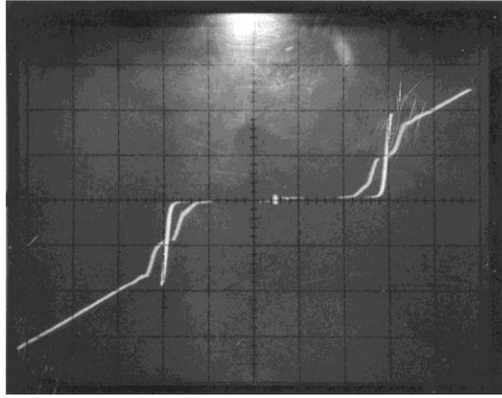
Figure 3. Mixer I-V pumped and un-pumped curves. The horizontal scale is 1 mV/div; the vertical one is 0.1 mA/div.
