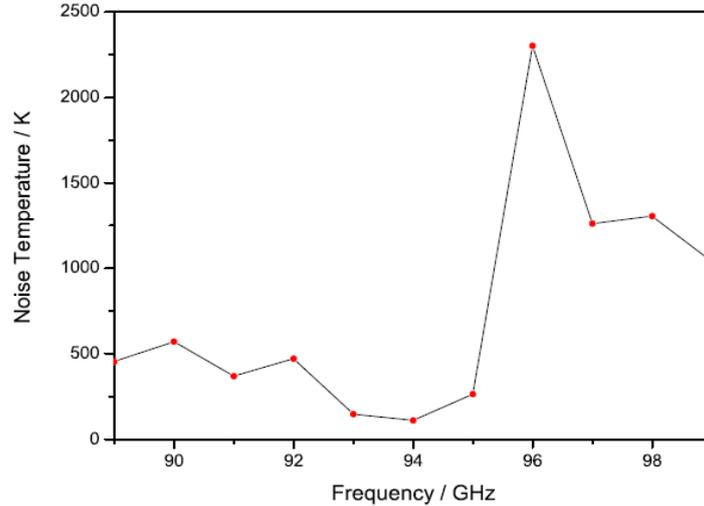
Figure 5. Preliminary results of the noise temperature of the MASTER 94 GHz prototype receiver. A colour version of the graph can be found in the on-line version of the paper.
