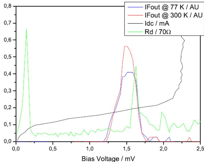
Figure 6. IF output hot and cold load down-converted signals, junction DC I-V characteristic and dynamic resistance (scaled by a factor of 70 to fit the graph scale). A colour version of the graph can be found in the on-line version of the paper.
