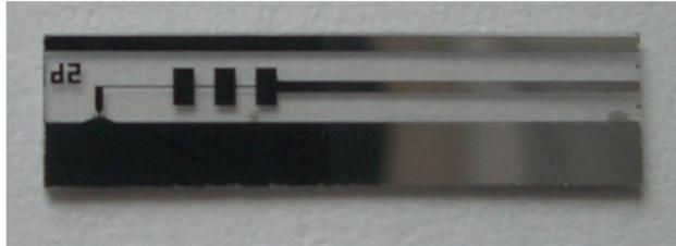
Figure 1. Picture of the MASTER 94 GHz SIS mixer chip.
