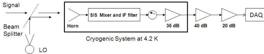
Figure 2. Schematization of the 94 GHz MASTER receiver.
