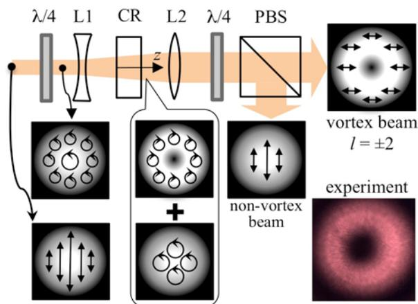
**Fig. 1.** Setup for the generation of double-charge femtosecond vortex pulses.  $\lambda/4$  – achromatic quarter-wave plate, L1 – negative lens, CR – uniaxial crystal, L2 – positive lens, PBS – polarization beamsplitter. Polarization states after each optical element are indicated by arrows. Bottom right: CCD image ( $4.2 \times 4.2 \text{ mm}^2$ ) of a double-charge vortex recorded  $\sim 5$  meters after the converter.
