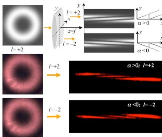
**Fig. 2.** Diagnostics of femtosecond vortex beam after the converter in Fig. 1: evidence of its singular nature and determination of the topological charge. Top: simulated behavior of a double-charge vortex at the focus of a positive cylindrical lens. Bottom: experimentally obtained images of femtosecond double-charge vortices 0.5 m after the converter (left) and their focal caustics (right). Horizontal size of all experimental images is 4.2 mm.
