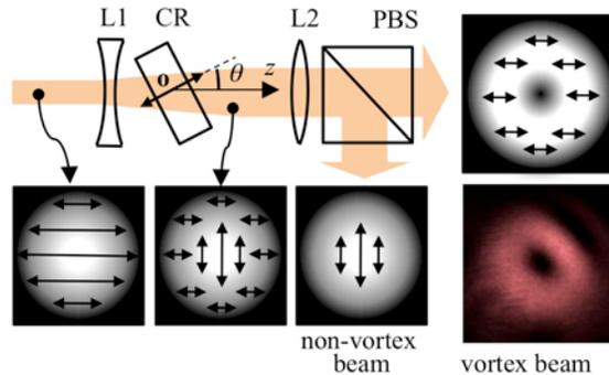
**Fig. 3.** Experimental set-up for the generation of double-charge femtosecond vortex pulses (the notations are as in Fig.1).  $\bullet$  denotes the optical axis of the crystal. Bottom right: CCD image ( $4.2 \times 4.2 \text{ mm}^2$ ) of a single-charge vortex recorded  $\sim 5 \text{ m}$  after the converter.
