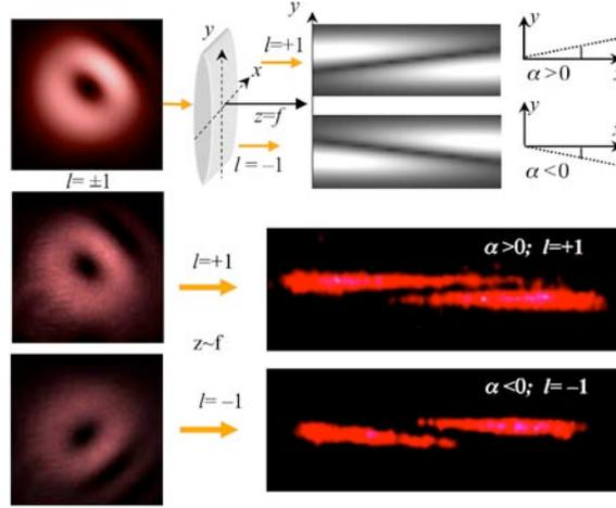
**Fig. 4.** Diagnostics of femtosecond vortex beam after the converter in Fig. 3: evidence of its singular nature and determination of the topological charge. Top: simulated behavior of a single-charge vortex at the focus of a positive cylindrical lens. Bottom: experimental images of femtosecond single-charge vortices 0.5m after the converter (left) and their focal caustics for the opposite topological charges (right). Horizontal size of all experimental images is 4.2 mm.
