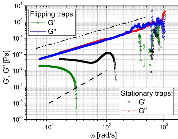
**Figure 5.** Storage ( $G'$ ) and loss ( $G''$ ) moduli of water *vs.* frequency, analysed using both Eq. (7) (high frequencies) and Eq. (10) (low frequencies) applied directly to the experimental data presented in Fig. 2 and Fig. 4, respectively. The lines represents the expected limiting behaviour of the moduli when the material reaches the terminal region:  $G' \propto \omega^2$  and  $G'' \propto \omega$ .
