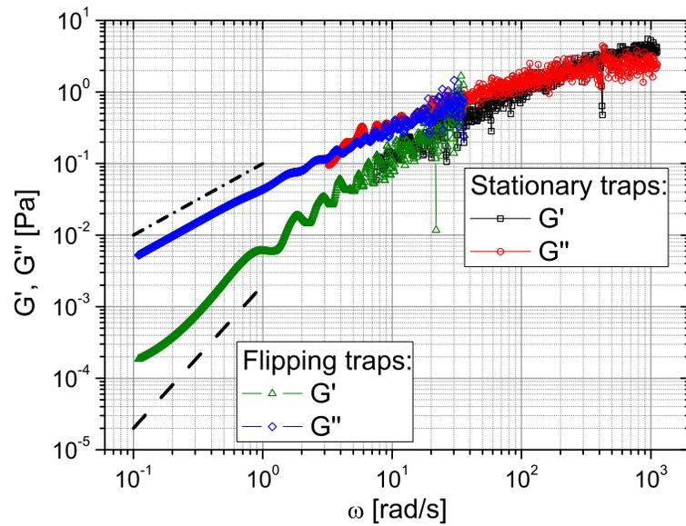
**Figure 6.** Storage ( $G'$ ) and loss ( $G''$ ) moduli *vs.* frequency of a solution of 1% w/w of PAM in water measured by means of both Eq. (7) (high frequencies) and Eq. (10) (low frequencies) applied directly to the experimental data presented in Fig. 2 and Fig. 4, respectively. The lines represents the expected limiting behaviour of the moduli when the material reaches the terminal region:  $G' \propto \omega^2$  and  $G'' \propto \omega$ .
