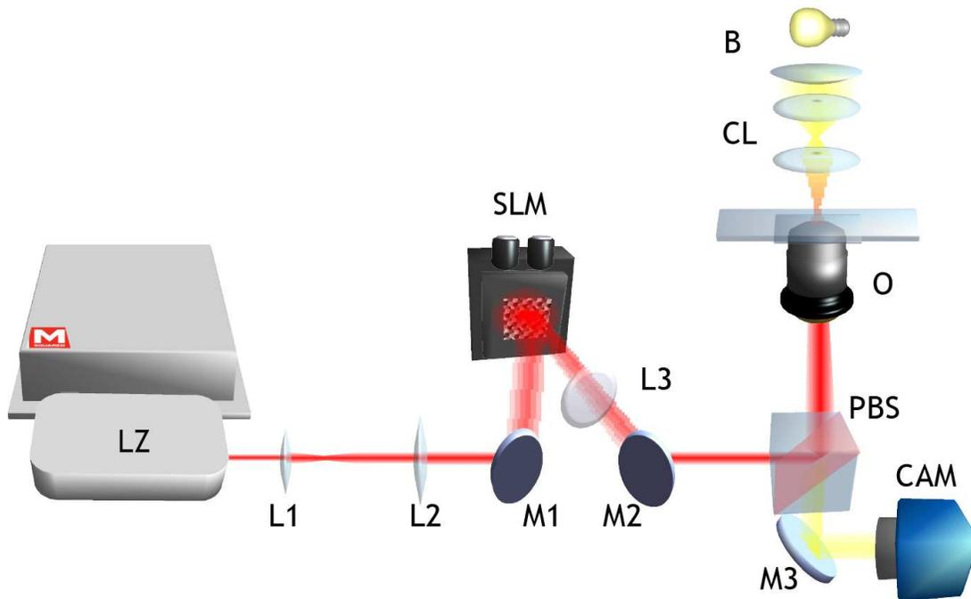
**Figure 1.** Experimental setup. From left to right. (LZ) Ti:sapphire laser system, (L1 and L2) Beam Telescope, (M1 and M2) Folding Mirrors, (SLM) Boulder Fast SLM, (L3), (PBS) Polarising beam splitter cube, (M3) Mirror, (CAM) Prosilica Fast camera, (O) Objective lens, (CL) Condensing optics, (B) 250W halogen bulb.
