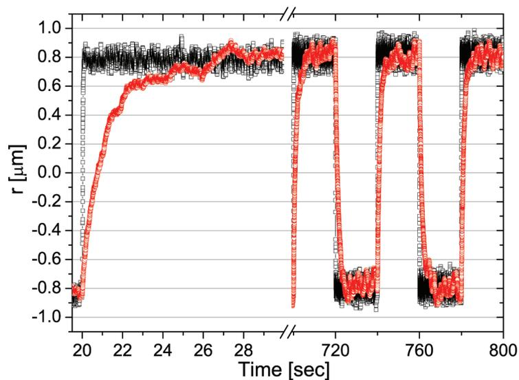
**Figure 3.** The trajectory of a  $5\mu\text{m}$  diameter bead flipping between two optical traps  $\kappa_1$  (bottom) and  $\kappa_2$  (top) repeatedly switching after a duration  $P = 20$  s. The bead is suspended in (squares) water (with  $\kappa_1 = 2.7$  and  $\kappa_2 = 2.5\mu\text{N}/\text{m}$ ) and (circles) a water-based solution of PAM at concentrations of 1 % *w/w* (with  $\kappa_1 = 2.1$  and  $\kappa_2 = 2.2\mu\text{N}/\text{m}$ ).
