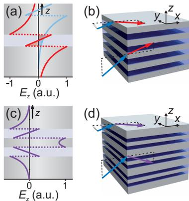
FIG. 3: (color) (a)  $E_z(z)$  profile of the antisymmetric mode in a MDM waveguide (red), together with  $E_z(z-d)$  (blue). (b) Refraction into an array of MDM waveguides. Arrows depict the direction of energy flow. (c)  $E_z$  profile of the backwards symmetric mode in a pair of MDM waveguides. (d) Refraction into an array of strongly coupled MDM waveguide pairs.
