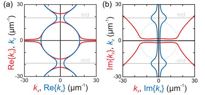
FIG. 7: (Supplemental). Calculated wavevector diagrams for the example structure described in the main text, including absorption in the Ag, taking either  $k_x$  or  $k_z$  to be complex. (a)  $\text{Re}(k_x)$  as a function of real  $k_z$  (blue) and  $\text{Re}(k_z)$  as a function of real  $k_x$  (red). (b)  $\text{Im}(k_x)$  as a function of real  $k_z$  (blue) and  $\text{Im}(k_z)$  as a function of real  $k_x$  (red). The grey dotted curves represent  $k_x^2 + k_z^2 = k_0^2$ .
