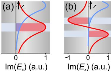
FIG. 6: (Supplemental). (a) Field profile of longitudinal electric field  $E_x(z)$  of the antisymmetric mode in a MDM waveguide (red), as well as the displaced field  $E_x(z-d)$  (blue), having positive overlap. (b) Profiles of  $E_x(z)$  (red) and  $E_x(z-d)$  (blue) of the symmetric mode in a pair of waveguides in the backwards wave regime, with a negative overlap.
