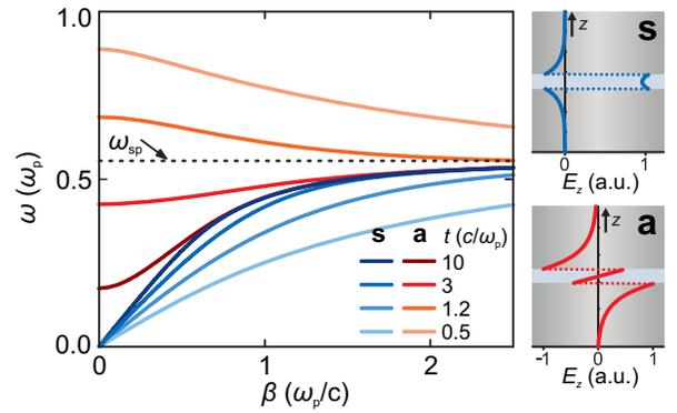
FIG. 2: (color) Dispersion in MDM waveguides for varying dielectric thickness  $t$ , showing the appearance of backwards SPPs for small  $t$ . On the right, characteristic  $E_z$  profiles of the symmetric (s) and antisymmetric (a) SPP modes are displayed.
