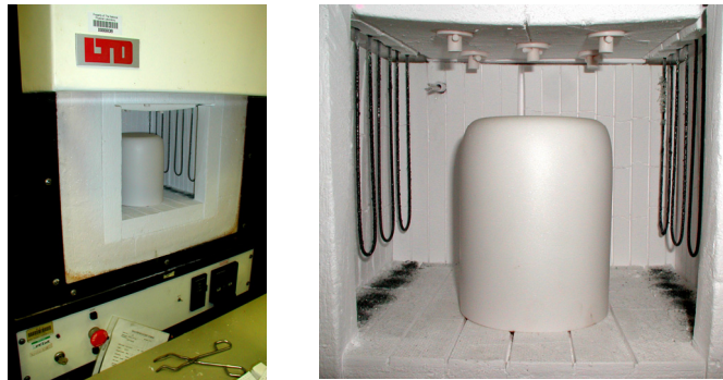
Fig. 1: Lenton chamber furnace for sapphire annealing
