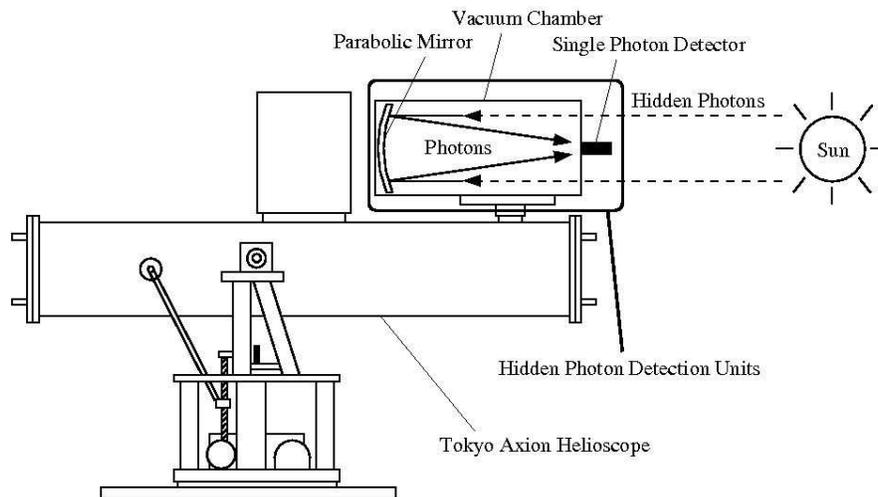
**FIGURE 3.** The schematic view of the apparatus to search for hidden photons from the sun.
