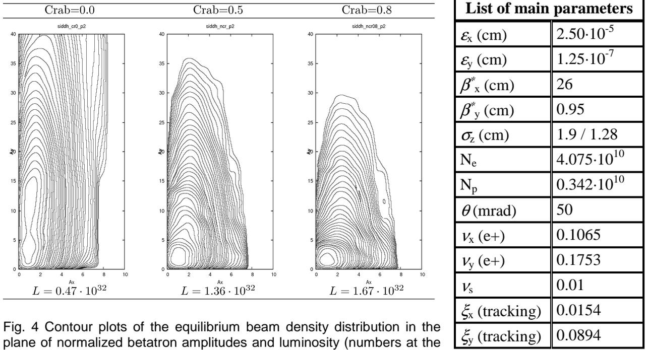
Fig. 4 Contour plots of the equilibrium beam density distribution in the plane of normalized betatron amplitudes and luminosity (numbers at the bottom) versus the crab sextupoles strength.
