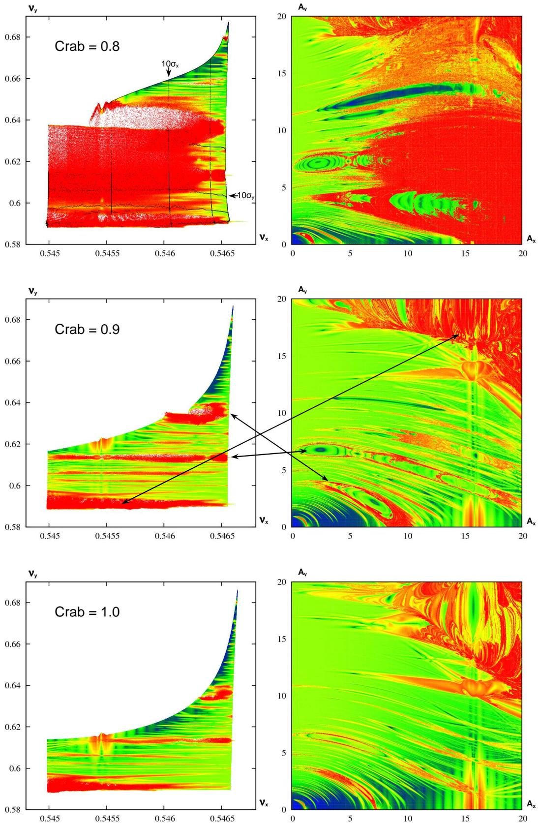
Fig. 10 Beam-beam resonances versus the crab value for SuperB LER.
