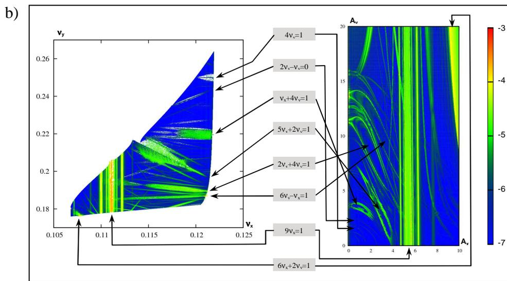
Fig. 5 Beam-beam resonances in the tune and amplitude planes for Crab=0.4. Correspondence between color and diffusion index is shown in the color palette on the right. In the case b) the diffusion index was calculated from the horizontal tune spread only.
