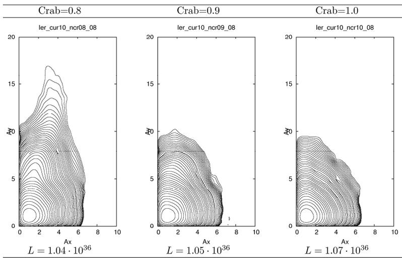
Fig. 9 Contour plots of the equilibrium beam density distribution for SuperB LER and luminosity (numbers at the bottom) versus the crab sextupoles strength.
