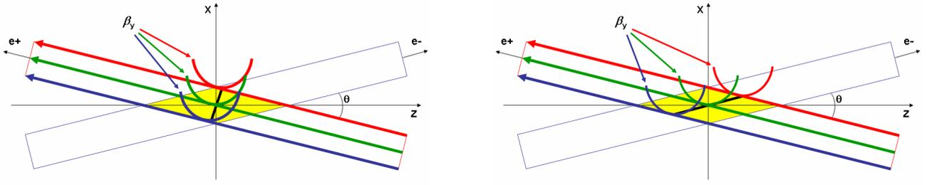
Fig. 2 Vertical beta function at IP without (on the left) and with the CW transformation.
