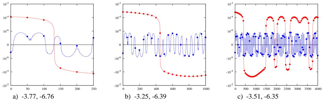
Fig. 3 Betatron tune deviation versus window shift for chaotic (red) and regular (blue) trajectories in different time scales. The diffusion indexes calculated from the bold dots are shown at the bottom.
