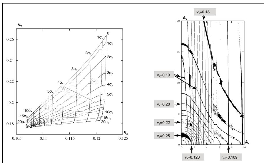
Fig. 6 Transformation between betatron tunes and betatron amplitudes.
