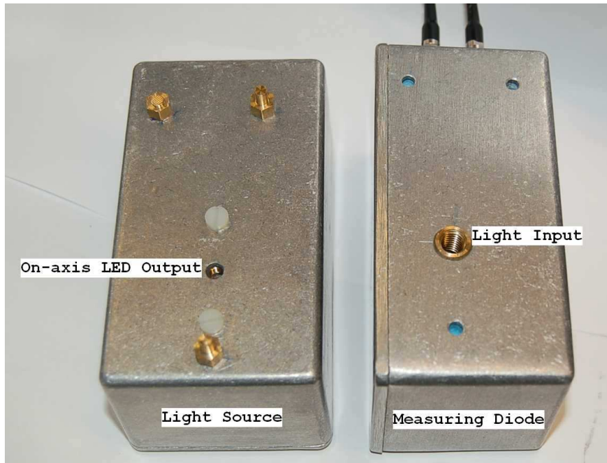
Figure 9. Photography of LED source (left) and monitoring system (right). Locating pins (yellow brass on left box) and boreholes (in blue on the right module) ensure reproducible positions of light-source and monitoring photo-diode
