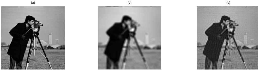
FIG. 5.2. Using MSA to solve (5.7). (a): Original image; (b): Blurred image; (c): Reconstructed image by MSA
