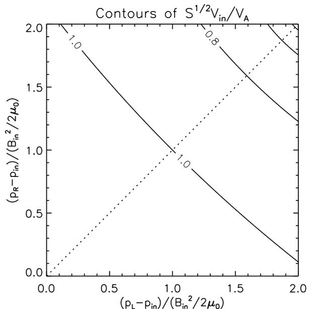
**Figure 3.** Contours of the normalized reconnection rate, given by  $S^{1/2}V_{in}/V_A = \sqrt{(V_L + V_R)/2V_A}$ , as a function of  $p_L - p_{in}$  and  $p_R - p_{in}$  and calculated using equation (29) to find  $V_L$  and  $V_R$  for the incompressible case. Contours are separated by 0.2.
