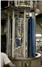
Fig. 7: Voltage multiplier in the ArDM experiment
