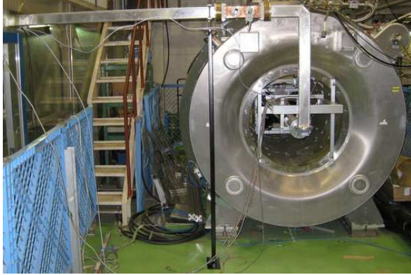
(a) The large bore superconducting magnet and the microwave waveguide. Microwaves are guided through the waveguide into the cavity.
