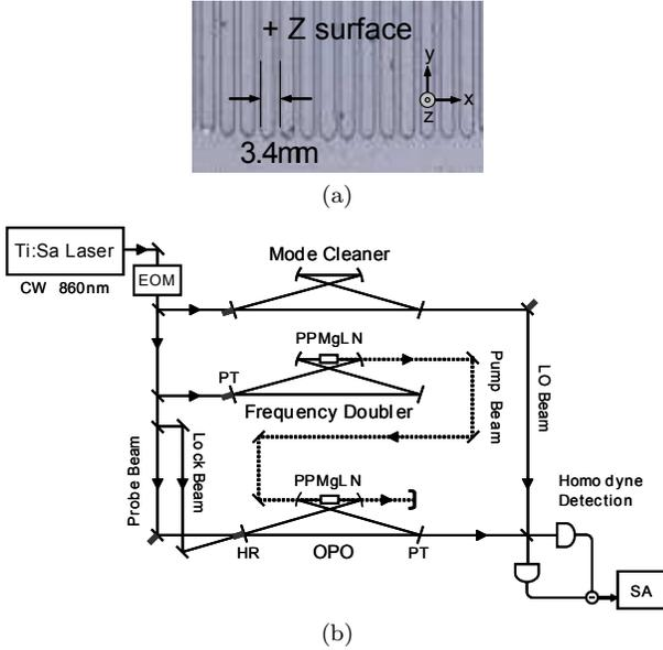
FIG. 1: (a) Observations of a periodically poled structure at +Z surface where an electrode was attached. (b) Schematic diagram of experimental setup.
