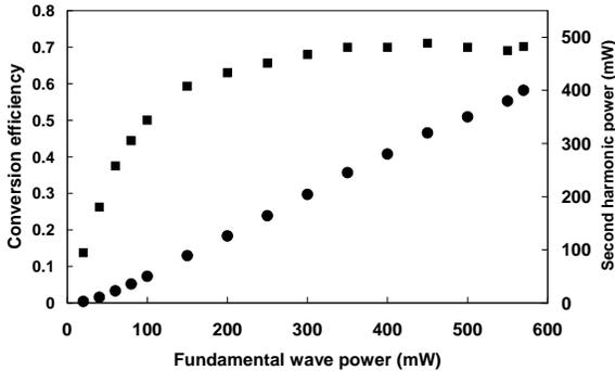
FIG. 2: A property of frequency doubler with the PPMgLN crystal. Circles and squares indicate the power of second harmonic wave at 430 nm and the conversion efficiency respectively.
