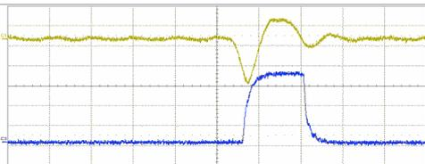
Figure 7 : fast shaper and discriminator outputs
