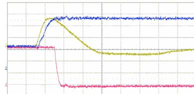
Figure 10 : slow shaper, trigger delayed and shaper hold signals
