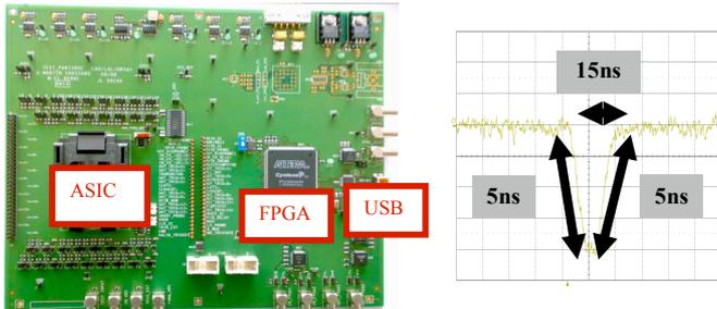
Figure 6 : Test board photography and input signal shape
