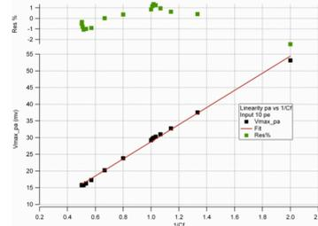
Figure 9 : preamplifier gain linearity
