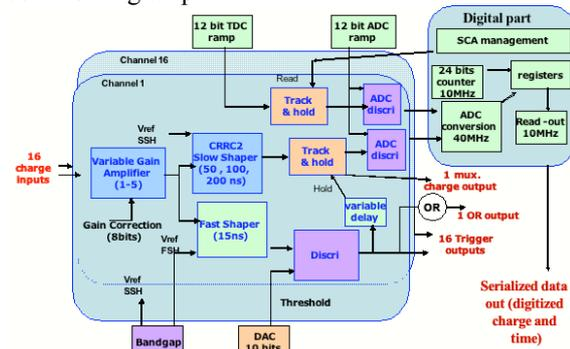
Figure 2: PARISROC global schematic
