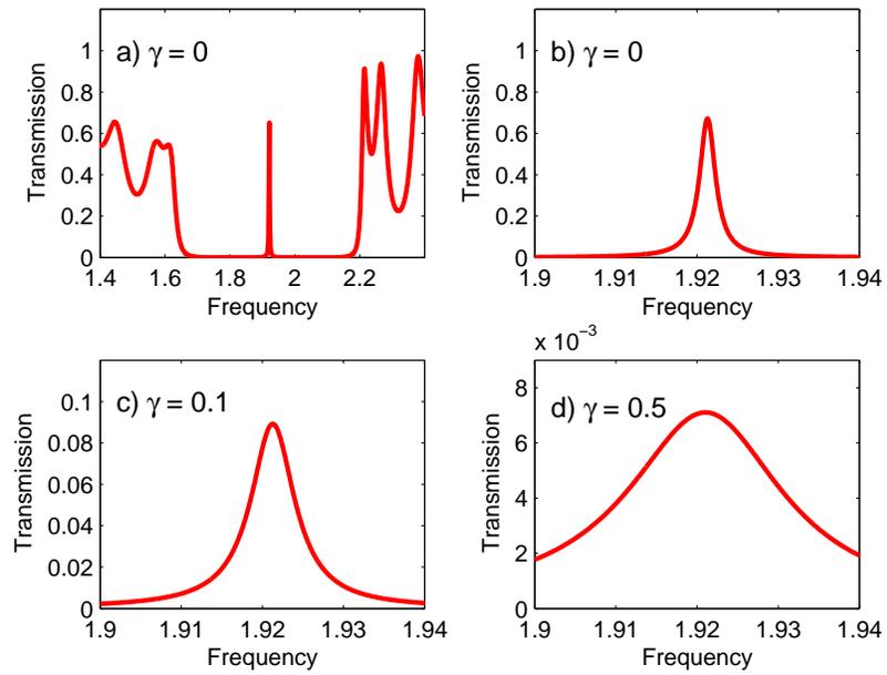
**Figure 3.** (Color online) Transmission dispersion of the layered array in Fig. 1 for different values of absorption coefficient  $\gamma$  of the D-layer. Circular birefringence  $\alpha$  is negligible. Fig. (b) shows the enlarged portion of Fig. (a) covering the vicinity of microcavity resonance.
