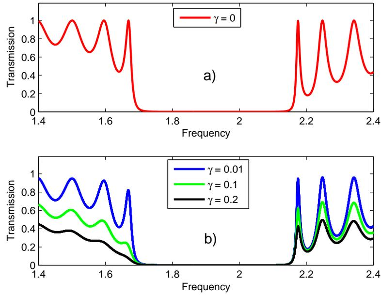
**Figure 7.** (Color online) Transmission dispersion of periodic layered structure in Fig. 2 for different values of absorption coefficient  $\gamma$  of the F-layers. Circular birefringence  $\alpha$  is negligible.
