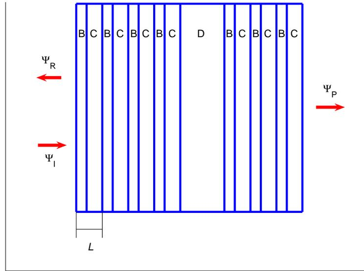
**Figure 1.** (Color online) Magnetic resonance cavity composed of magnetic layer D sandwiched between a pair of identical periodic non-magnetic stacks (Bragg reflectors). The incident wave  $\Psi_I$  is linearly polarized with  $E \parallel x$ . Due to the nonreciprocal circular birefringence of the magnetic material of D-layer, the reflected wave  $\Psi_R$  and the transmitted wave  $\Psi_P$  are both elliptically polarized.
