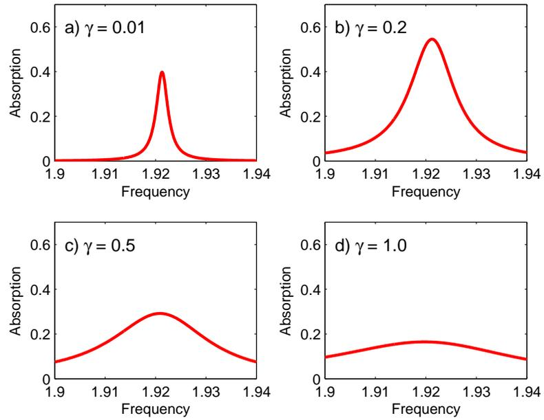
**Figure 5.** (Color online) Frequency dependence of absorption of the layered array in Fig. 1 for different values of absorption coefficient  $\gamma$  of the D-layer. Circular birefringence  $\alpha$  is negligible. The frequency range shown covers the vicinity of microcavity resonance. Observe that the stack absorption decreases after coefficient  $\gamma$  exceeds certain value, which is in sharp contrast with the case of a periodic stack, shown in Figs. 8.
