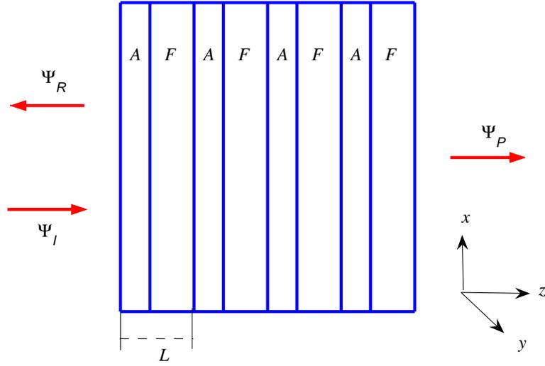
**Figure 2.** (Color online) Periodic layered structure composed of alternate magnetic (F) and dielectric (A) layers. The F-layers are made of the same lossy magnetic material as the D-layer in Fig. 1.  $L$  is the unit cell length. The incident wave  $\Psi_I$  is linearly polarized with  $E \parallel x$ . Due to the nonreciprocal circular birefringence of the magnetic material of the F-layers, the reflected wave  $\Psi_R$  and the transmitted wave  $\Psi_P$  are both elliptically polarized.
