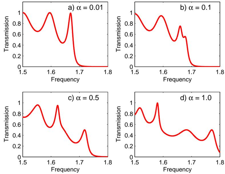
**Figure 10.** (Color online) Transmission dispersion of periodic layered structure in Fig. 2 for different values of circular birefringence  $\alpha$  of the F-layers and zero absorption. When circular birefringence  $\alpha$  is large enough, each transmission resonance splits into a pair of twin resonances, corresponding to two circularly polarized modes with opposite sense of rotation. The incident wave polarization is linear.
