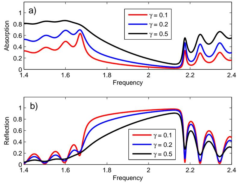
**Figure 8.** (Color online) Frequency dependence of (a) absorption and (b) transmission of periodic layered structure in Fig. 2 for different values of absorption coefficient  $\gamma$  of the F-layers. Circular birefringence  $\alpha$  is negligible.
