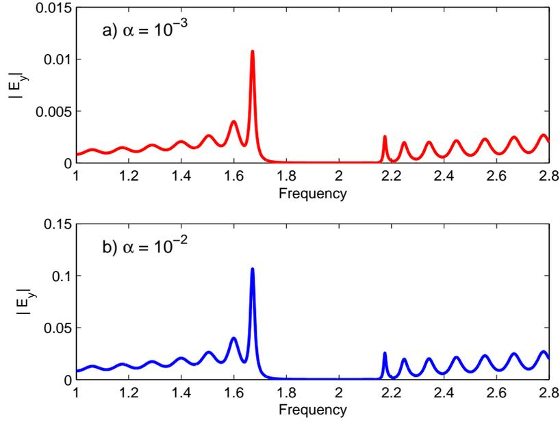
**Figure 9.** (Color online) Frequency dependence of polarization component  $|E_y|$  of the wave transmitted through the periodic layered structure in Fig. 2 for different values of circular birefringence  $\alpha$  of the F-layers and zero absorption. The incident wave is linearly polarized with  $\vec{E} \parallel x$ .
