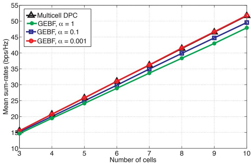
Fig. 4. Sum-rates as a function of the number of cells ( $K$ ) for  $\alpha = \{0.001, 0.1, 1\}$ , when  $N_t = 4$ ,  $\rho_{(d)} = 10$  dB, for GEBF with full CSI.
