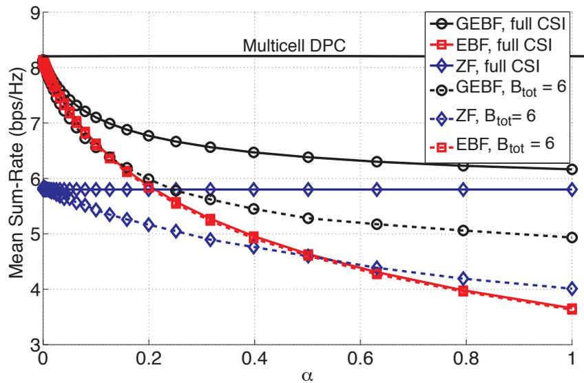
Fig. 6. Comparison of the mean sum-rates obtained using the proposed beamforming strategy, non-cooperative eigenbeamforming and (cooperative) zero forcing, for  $\rho_{(d)} = 10$  dB,  $N_t = K = 2$  and  $B_{\text{tot}} = 6$ .
