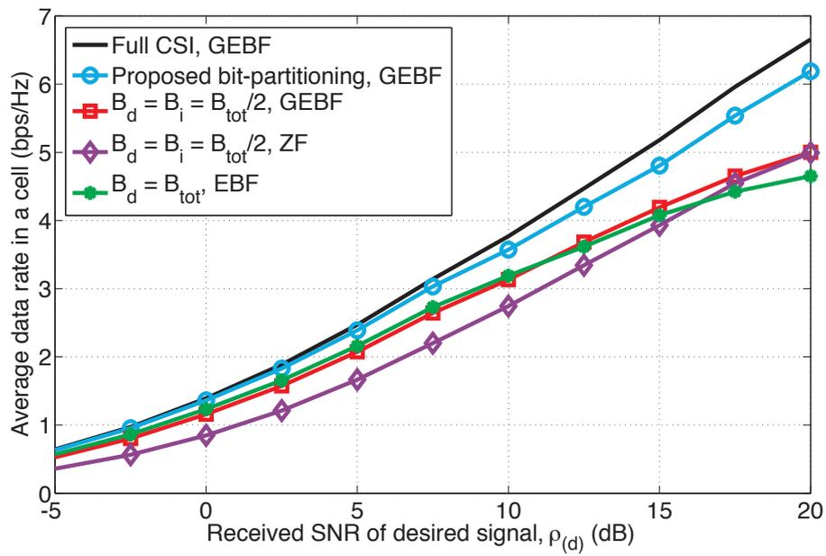
Fig. 9. Average data rate in a cell as a function of the received desired signal power for  $N_t = K = 2$  and  $B_{tot} = 6$ .
