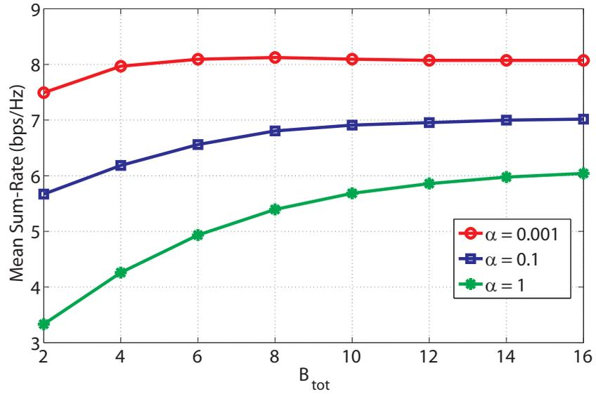
Fig. 7. Comparison of the mean sum-rates obtained using GEBF for  $\alpha = \{0.001, 0.1, 1\}$  as a function of  $B_{\text{tot}}$ , for  $\rho_{(d)} = 10 \text{ dB}$ ,  $N_t = K = 2$ .
