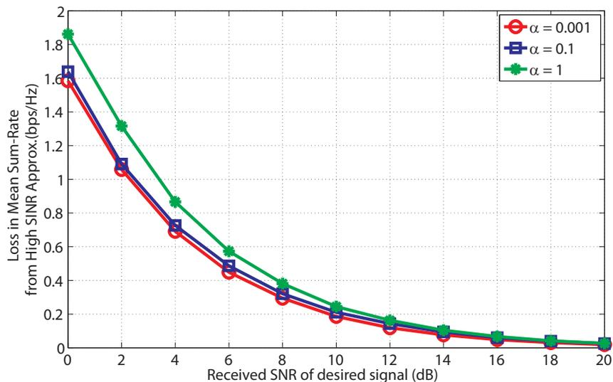
Fig. 3. Comparison of the actual and high SINR approximated sum-rates (in (4) and (7), respectively) for  $\alpha = \{0.001, 0.1, 1\}$ , when  $N_t = 4$ ,  $\rho_{(d)} = [0, 20]$  dB and  $K = 4$  for full CSI.
