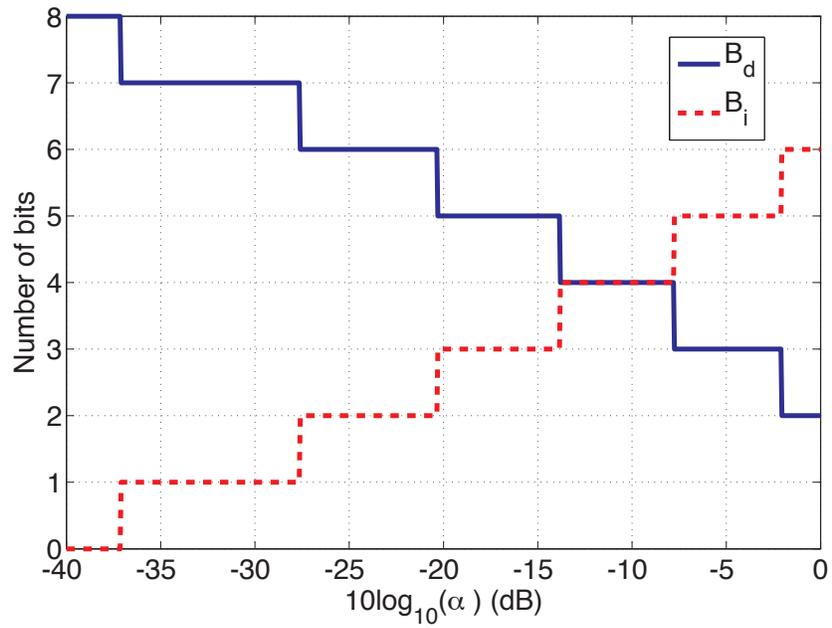
Fig. 8.  $(B_d, B_i)$  partitioning for, for  $\rho_{(d)} = 10 \text{ dB}$ ,  $N_t = K = 2$  and  $B_{\text{tot}} = 8$ .
