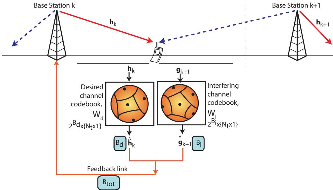
Fig. 2. The limited feedback model, described in Section IV, to feedback quantized CSI of the desired and interfering channels using two separate codebooks.
