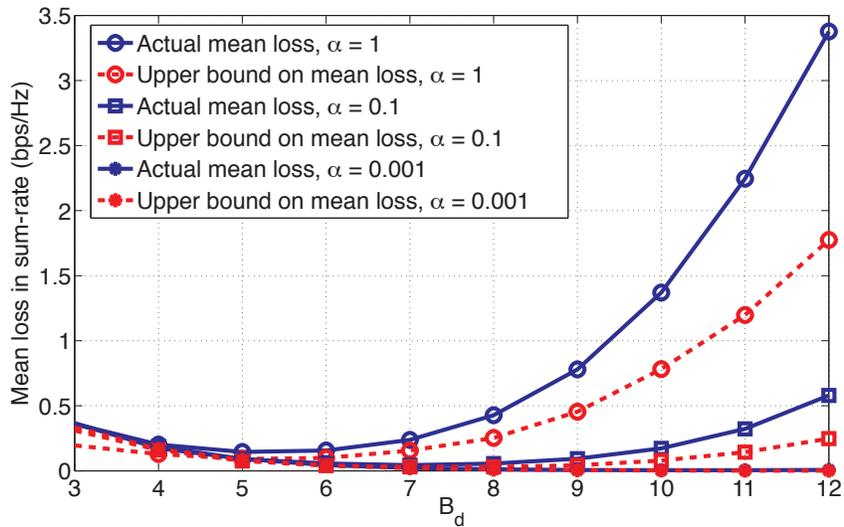
Fig. 5. Mean loss in sum-rate for  $\alpha = \{10.001, 0.1, 1\}$ ,  $N_t = K = 2$ ,  $\rho_{(d)} = 10$  dB and  $B_{\text{tot}} = 15$ .
