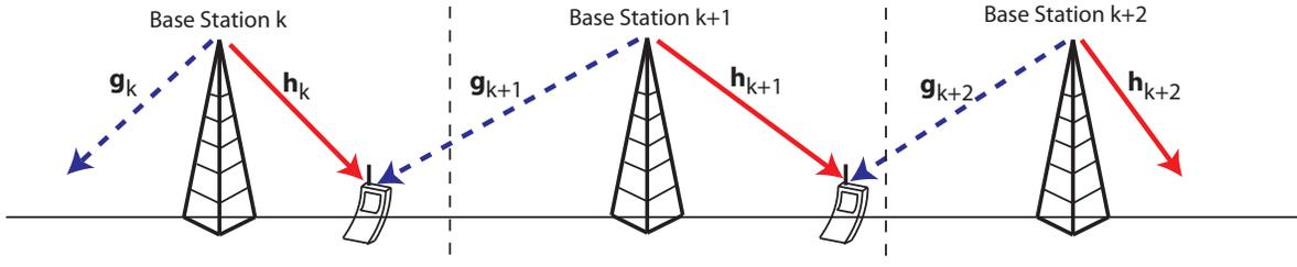
Fig. 1. Pictorial depiction of the Wyner model (described in Section II). The solid line represents the desired signal, while the dashed line represents the interfering signal.
