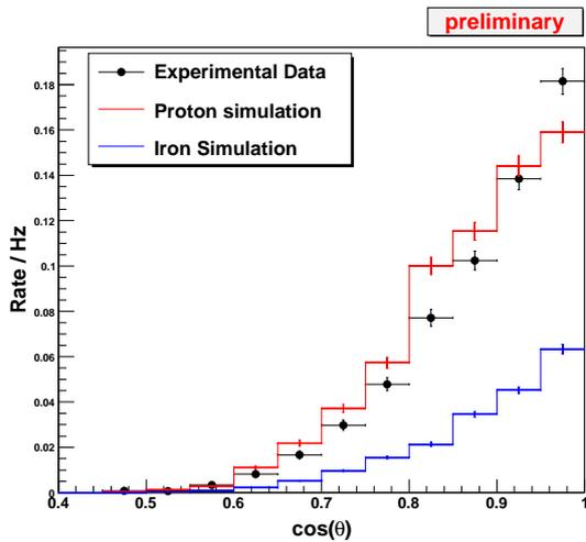
Fig. 6: Reconstructed zenith distributions for 3 station events.
