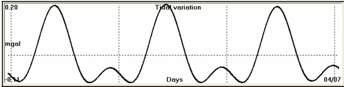
Fig. 10. Three day's sample of the tidal variation. The vertical scale is expressed in mgals since the related computer code was addressing the problem of tidal corrections (vertical component) in gravity surveys.
