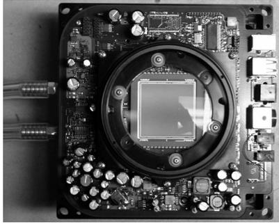
Figure 1. Custom-designed FLI CCD with field flattener.
