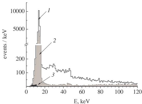
FIG. 6: Amplitude spectra (1) of single-, (2) two-point, and (3) three-point events that form the total analyzed pulse amplitude spectrum of the counter detecting both background and  $^{81}\text{Kr}$  decays.
