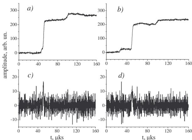
FIG. 4: Primary ionization signals for two types of two-point energy deposits from K-capture of  $^{81}\text{Kr}$  isotope accompanied by an escape of a characteristic photon and a concomitant Auger electron: (a, b) recalculated voltage (charge) pulses and (c, d) corresponding current pulses from primary ionization electrons.
