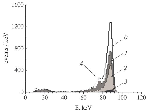
FIG. 2: Pulse amplitude spectrum from the external <sup>109</sup>Cd source located in the middle of the LPC length: (0) all events, (1) single-point events, (2) two-point events, (3) three-point events, and (4) escape peak of characteristic  $\gamma$ -ray photons.
