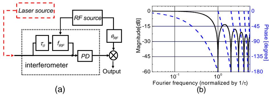
Fig.1. (a) Heterodyne interferometer, PD (Photodiode); (b) transfer function of the interferometer: relative magnitude  $|T(f)|/2\pi\tau_0$  [black solid line] and phase [blue dashed line] of frequency response of the interferometer.
