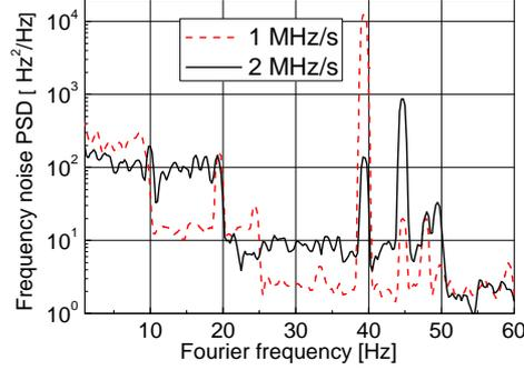
Fig. 6. Frequency noise power density of chirped laser at different chirping rates (a linear frequency drift is removed).
