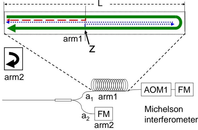
Fig. 1-1. The RBS effect on the laser frequency: AOM modulated reference signal (wide green line in arm1), short arm reference signal (wide black one), the RBS signals (red dash line, blue dot line);  $a_1$  and  $a_2$  are field amplitude coupling coefficients from the common input (in power).
