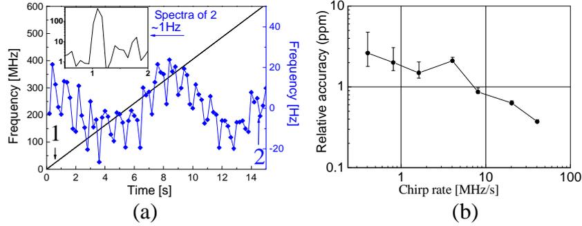
Fig. 9. (a-1) Beat-note signal frequency of the chirped laser vs. ULE-cavity stabilized laser, (a-2) residual frequency fluctuations (0.2 s gate time) after removing linear frequency fit (blue line+diamonds), (insert) the PSD of the residuals of a-2, (b) chirp rate accuracy with respect to the chirp rate.
