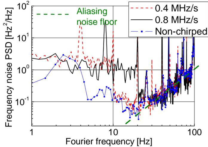
Fig. 8. Frequency noise of single RBS suppressed fiber-stabilized laser for various chirp rates.
