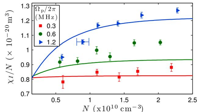
FIG. 5. (Color online). Cooperative non-linearity measured for  $|r\rangle = 42S_{1/2}$ , showing strong density dependence at high probe field. The interactions increase rapidly with  $N$  due to the  $1/R^6$  scaling, causing the susceptibility to plateau as  $V > \Omega_c$ . Solid lines show model integrated over nearest neighbour distribution.
