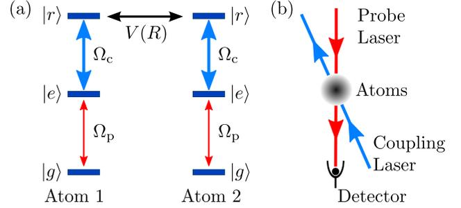
FIG. 1. (Color online). (a) Pair model for interacting three-level atoms. States  $|g\rangle$ ,  $|e\rangle$  and  $|r\rangle$  are coupled by a probe field  $\Omega_p$  and a strong coupling field  $\Omega_c$ . Dipole-dipole interactions couple the Rydberg states with strength  $V(R)$ . (b) Schematic of experiment. EIT spectroscopy is performed on an ultracold  $^{87}\text{Rb}$  atom cloud.
