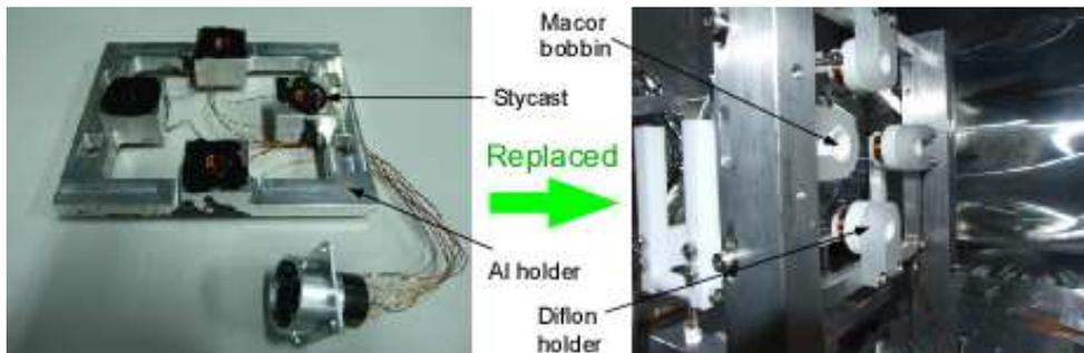
**Figure 6.** Photographs of coil holders; Left: The previous coil-holder. Coils are surrounded by a coil-holder made of aluminum, and fixed into the coil-holder using stycast. Right: The new coil-holder. Coils are wound on macor bobbins fixed on an aluminum frame through diflon holders.
