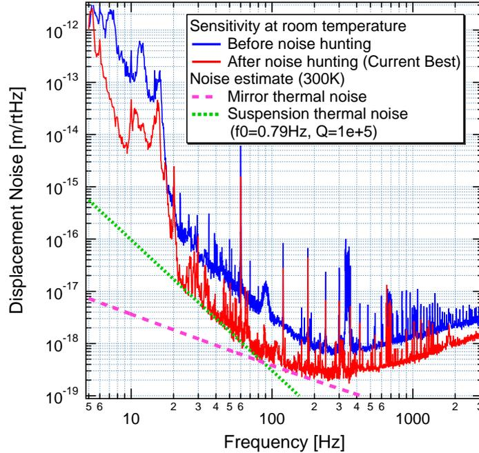
**Figure 2.** Improvement of the sensitivity in 2008; Solid lines of red and blue are the measured sensitivity after noise hunting (Current best) and before noise hunting, respectively. The green dotted line is the estimated suspension thermal noise from wire material dissipations using Q-factors of the violin modes. The pink dash line indicates the calculated mirror thermal noise due to the substrate of the thermoelastic damping.
