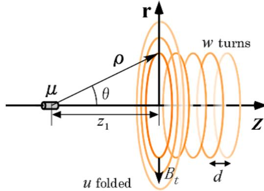
Figure 3. Model of a coil-magnet actuator
