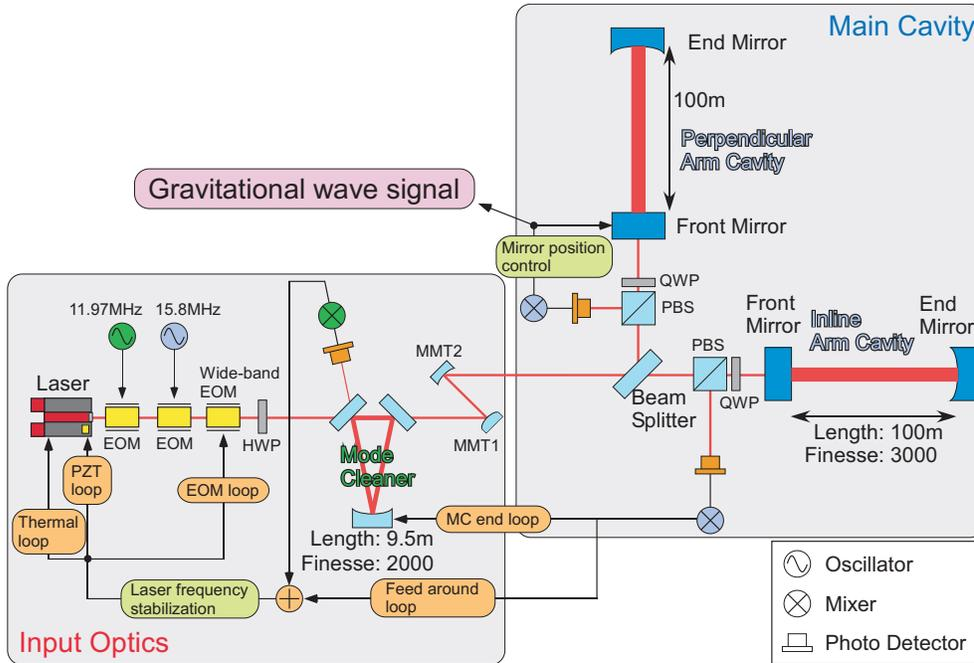
**Figure 1.** Schematic view of CLIO; CLIO is a so-called locked Fabry-Perot interferometer, which has two 100 m Fabry-Perot cavities with a mode cleaner. The optics, like the lenses, the Faraday-isolators, and some wave plates are omitted in this figure. Abbreviations denote: EOM, electro-optic modulator; HWP, half wave plate; QWP, quarter wave plate; MMT, mode matching telescope; and PBS, polarized beam splitter.
