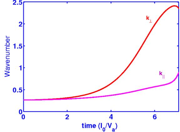
**FIGURE 2.** Evolution of  $\langle k_{\perp}(t) \rangle$  and  $\langle k_{\parallel}(t) \rangle$  as a measure of anisotropy in Hall MHD. Initially,  $\langle k_{\perp}(t=0) \rangle = \langle k_{\parallel}(t=0) \rangle$ . As time evolves, anisotropy in spectral transfer progressively develops such that  $\langle k_{\perp}(t) \rangle > \langle k_{\parallel}(t) \rangle$ .
