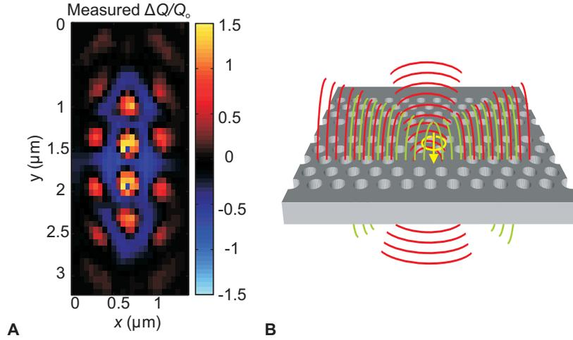
FIG. 6: **A**, Image of the measured shift of the quality factor  $\Delta Q/Q_0$  at every probe position. An increase and the decrease of the quality factor of the cavity is evident. **B**, Representation of the proposed mechanism that causes the increase of the quality factor. As the probe is above a maximum of the magnetic field, the induced current generates radiation that destructively interferes with the radiative loss of the cavity, yielding an increase of the photon lifetime.
