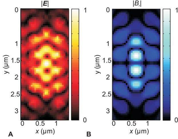
FIG. 4: **A** and **B**, Distribution of the magnitude of the electric field  $\mathbf{E}$  and of the amplitude of the vertical component of the magnetic field  $B_z$  normalized to their maximum, respectively. The area shown is the same as Fig. 3A. The two pictures show a different symmetry in the pattern of the field distributions.
