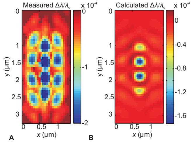
FIG. 5: **A** and **B**, Images of the measured and calculated shift of the resonance  $\Delta\lambda_0/\lambda_0$  at every probe position. Figure 5A shows an evident blue-shift of the resonance when the probe is above maxima of the  $|B_z|$ . We find an excellent quantitative agreement with the calculated resonance shift in Fig. 5B.
