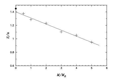
Figure 5: Stride lengths S, scaled with the length parameter a, for the motion in fluid with constant viscosity and fixed gait but a range of body masses. The crosses denote the SPH results and the filled circle denotes the result of Eldredge. The line of best-fit is also shown.
