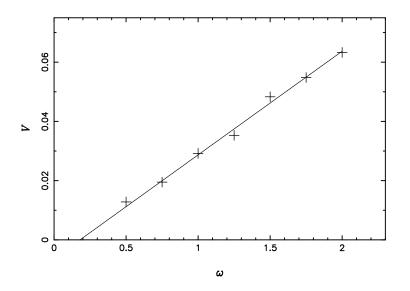
Figure 8: Velocity of the linked bodies for different frequencies with constant Reynolds number and amplitude. The SPH results are shown by the crosses and the continuous curve is a best fit straight line.
