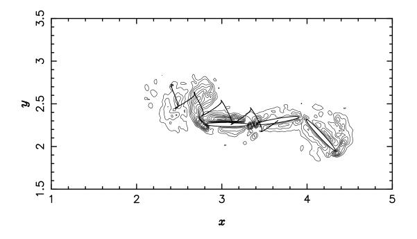
Figure 6: Vorticity field generated by the swimming linked bodies with  $M = 0.5M_0$ . This plot is at time  $t \sim 25$ . The vorticity contours have values in the range -5 to 5 with 40 levels. The stride path is also shown.
