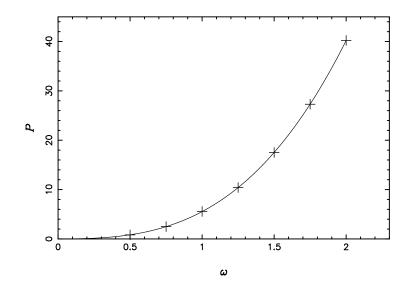
Figure 9: Power expended by the linked bodies for different frequencies with constant Reynolds number and amplitude. The SPH results are shown by crosses and the continuous curve is a best fit cubic.
