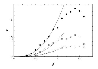
Figure 11: Velocity curves of constant viscosity and frequency against amplitude. Crosses, open circles and filled circles are for  $\omega = 0.75$ , 1.25 and 2.0 respectively. The curves are from (7.12), which is appropriate for  $\beta < 1$ .
