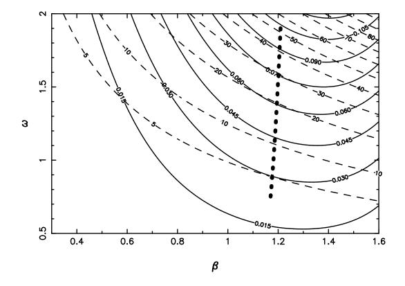
Figure 15: Velocity and average power contours on a frequency-amplitude plot. The solid lines are the velocity contours, and the dashed lines are the power contours. The thick dotted line is the curve of optimal motion.
