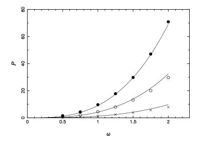
Figure 12: Average power curves of constant viscosity and amplitude against frequency. Crosses, open circles and filled circles are for  $\beta = 0.5$ , 0.9 and 1.3 respectively. The curves are from (7.14).
