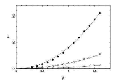
Figure 13: Average power curves of constant viscosity and frequency against amplitude. Crosses, open circles and filled circles are for  $\omega = 0.75$ , 1.25 and 2.0 respectively. The curves are from (7.14).
