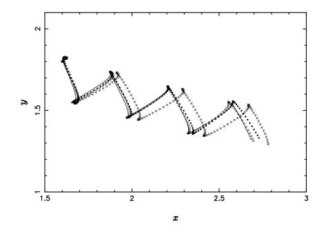
Figure 3: The stride paths for different resolutions. The crosses denote the stride path with dp = 1/30. Open circles, filled circles and the solid line are for dp = 1/40, 1/50 and 1/60 respectively.
