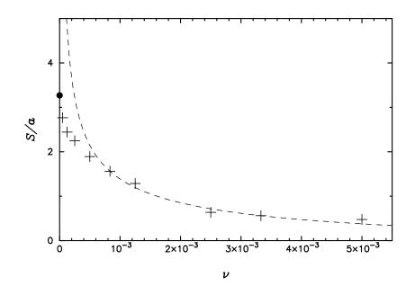
Figure 7: Stride lengths, in terms of length parameter a, for the motion in a fluid with different viscosities  $\nu$  but constant gait and mass. The crosses denote the SPH results and the filled circle denotes the result of Kanso et al. The dashed curve is based on an analytical result by Taylor, which is not expected to be valid for very high Reynolds number. Note that if  $\nu = 10^{-3}$  then Re = 250.
