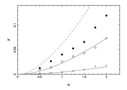
Figure 10: Velocity curves of constant viscosity and amplitude against frequency. Crosses, open circles and filled circles are for  $\beta = 0.5$ , 0.9 and 1.3 respectively. The curves are from (7.12) with constants fitted from the set with  $\beta = 0.9$ . The dashed curve is for  $\beta = 1.3$ , which is outside the range for which (7.12) is valid.
