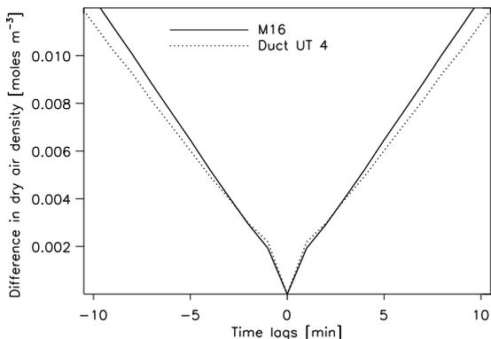
**Fig. 7** Square root of the temporal structure function of the dry air density at two locations in the VLTI for the Night 22/23 September 2004. The solid line shows the temporal structure function for measurements at the M16 mirror in front of the interferometric laboratory, and the dashed line displays the same measurements inside the light duct towards the UT 4 telescope.
