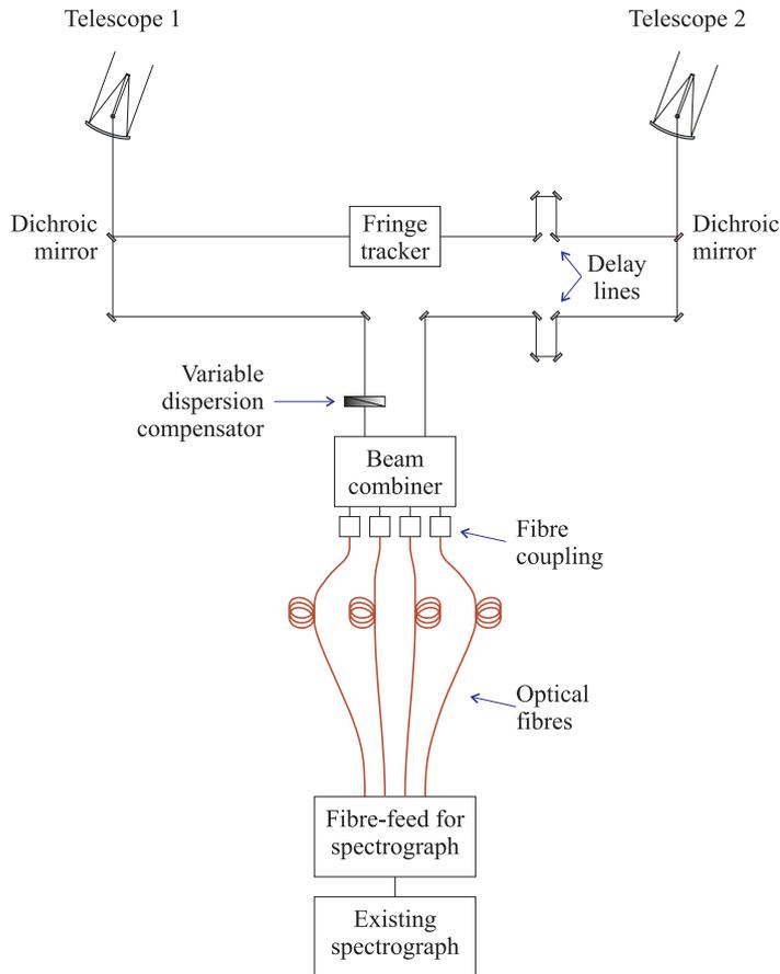
**Fig. 1** Schematic of the combined instrument, interferometer and spectrograph. The proposed instrument relies on pre-existing infrastructure (telescopes, fringe-tracker, delay lines and a spectrograph located within a few hundred meters). The additional components which must be built include the variable dispersion compensator, beam combiner, fiber coupling, optical fibers and fiber-feed for the spectrograph.
