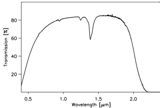
**Fig. 5** Transmission in the wavelength range from 0.4 to 2.5  $\mu\text{m}$  for 150 m of Optran Plus WF fiber (Ceramoptec catalog, see <http://www.ceramoptec.com/catalog.htm>).
