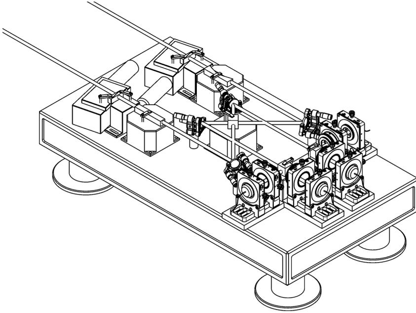
**Fig. 9** UVES-I beam combination table. The light beams from the two telescopes enter from the top left, and pass through the atmospheric dispersion compensator and achromatic phase shifter before being combined at the central beam combiner. The two polarization states are separated, and the resulting four beams coupled into optical fibers; the four fiber holders are visible at the bottom right.
