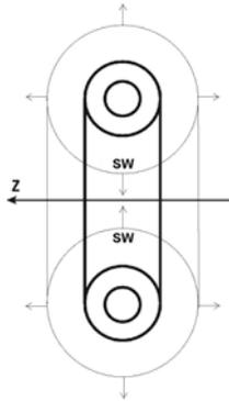
Registration of shadow pictures was carried out by means of the pulse ruby laser. Duration of a pulse is 20 ns. In Fig 1. is shown the a ring discharger and a laser beam direction.
