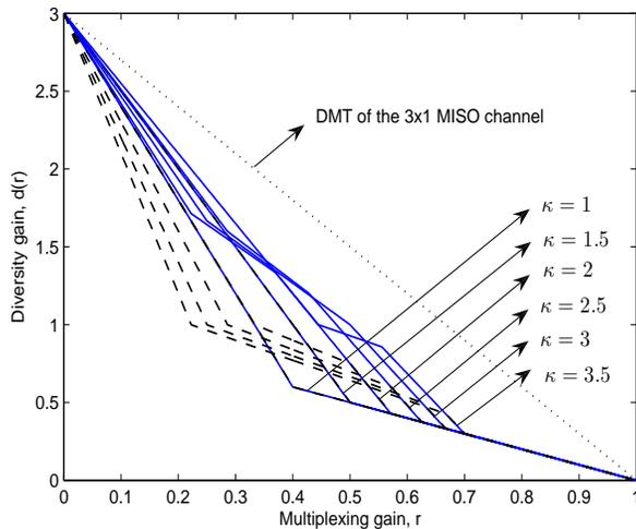
Fig. 4. The DMT performances of the asynchronous OSDF protocol over a two relay network for both finite and infinite length shaping waveforms and for various values of  $\kappa > 1$ .
