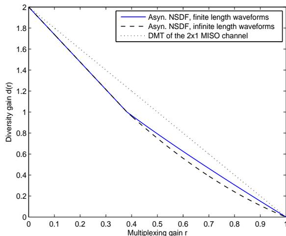
Fig. 3. The DMT performances of the asynchronous NSDF protocol over a single relay network for both finite and infinite length shaping waveforms and optimum values of  $\kappa > 1$ .
