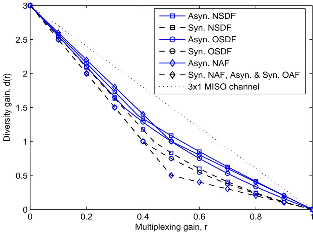
Fig. 9. DMT performance of the asynchronous protocols and the corresponding synchronous counterparts in a two relay network.
