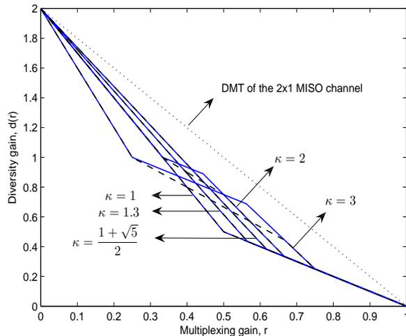
Fig. 2. The DMT performances of the asynchronous NSDF protocol over a single relay network for both finite and infinite length shaping waveforms and for various values of  $\kappa > 1$ .
