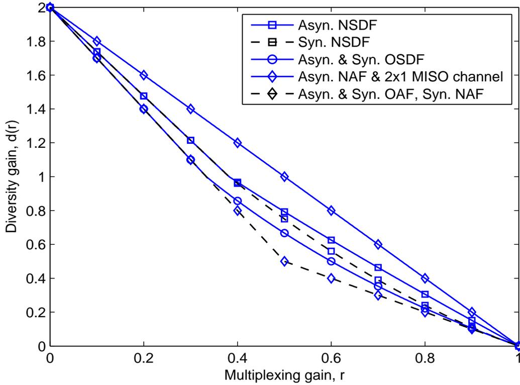
Fig. 8. The DMT performances of the asynchronous protocols and the corresponding synchronous counterparts in a single relay network.
