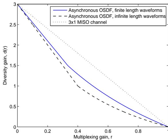
Fig. 5. The DMT performances of the asynchronous OSDF protocol over a two relay network for both finite and infinite length shaping waveforms and optimum values of  $\kappa > 1$ .
