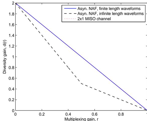
Fig. 6. The DMT performances of the asynchronous NAF protocol for both finite and infinite length shaping waveforms and optimum values of  $\kappa = 1$ .
