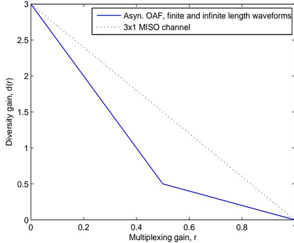
Fig. 7. The DMT performances of the asynchronous NSDF protocol for both finite and infinite length shaping waveforms and optimum values of  $\kappa$ .
