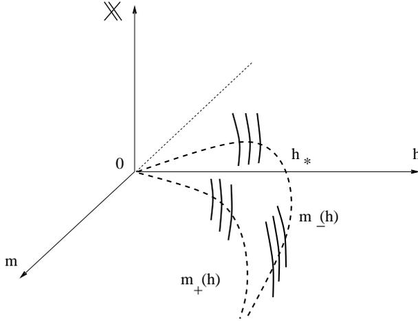
Figure 4. The case  $\gamma > 0$ : The dashed curves represent the laminar bifurcating flows .
