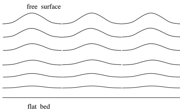
Figure 2. Flow pattern (streamlines) without stagnation points.
