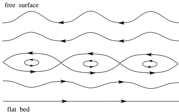
Figure 3. Flow pattern (streamlines) with stagnation points :
