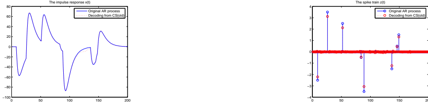
Figure 6: \ell_1 -minimization algorithm on the model y = Gx + w with G an 80 \times 200 Toeplitz Gaussian matrix ensemble. The filtered process x(n) is obtained by filtering a 8 sparse spike train through a third-order AR process with poles \alpha_1 = 0.9 , \alpha_2 = 0.5 and \alpha_3 = 0.2 . The measurements were contaminated with zero mean Gaussian noise with variance 0.1.
